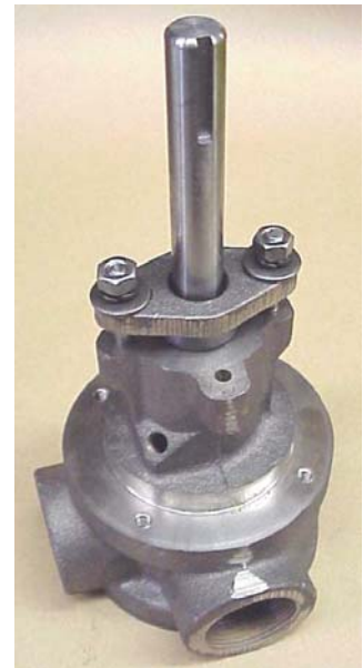
Figure 9, Gland & shaft installed
