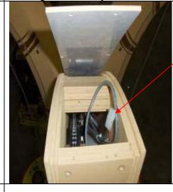
There should be two pigtails like this. One for the LED light and one for the beacon
