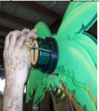
7) Mate LED plug and Beacon plug with corresponding mating plug in Palm Arch and wire tie them. They should be numbered.
