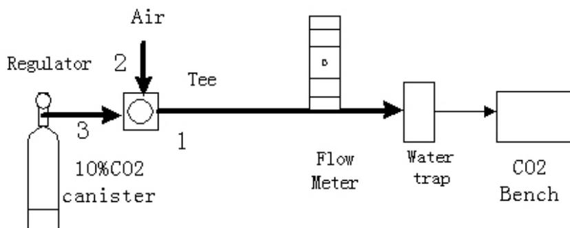
Figure 5-6 Sidestream test set up
