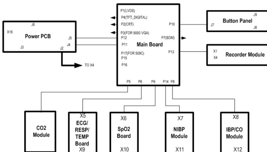
Figure 2-3 PCB connection
