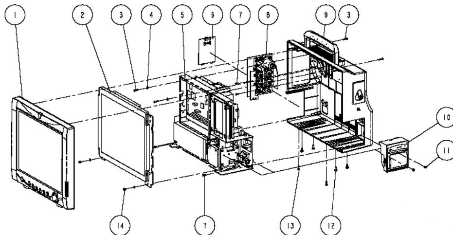
Figure 4-1 Exploded view of DPM5
