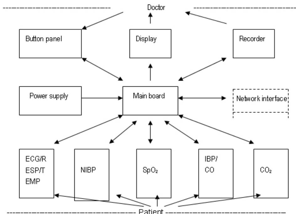
Figure 2-14 System structure
