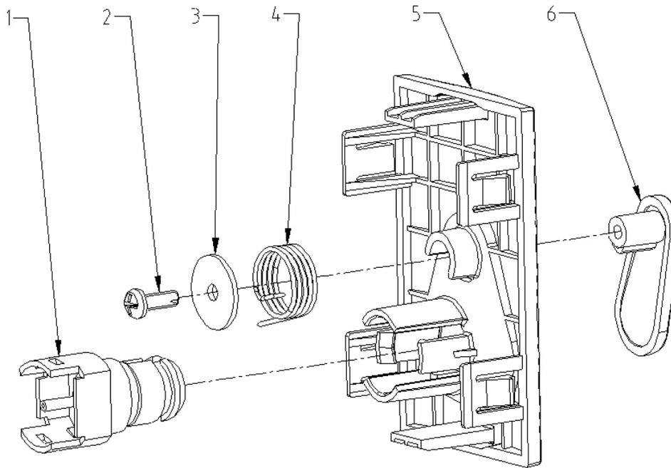
Figure 4-6 Microstream CO<sub>2</sub> assembly
