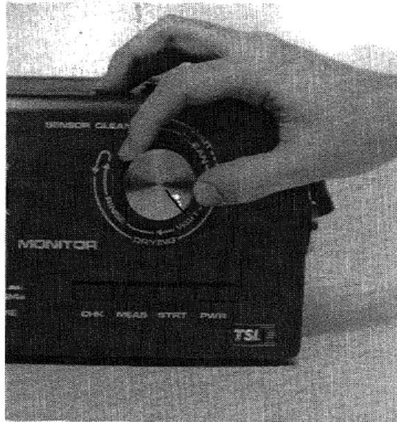
**Figure 23.** Sensor in the soak position
