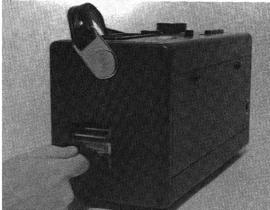
**Figure 10.** Removing the sponge compartment door
