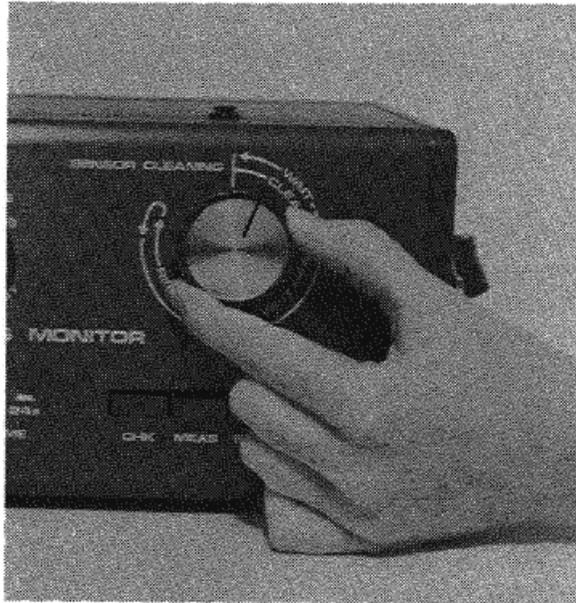
**Figure 25.** Sensor-cleaning dial turned 10 degrees
