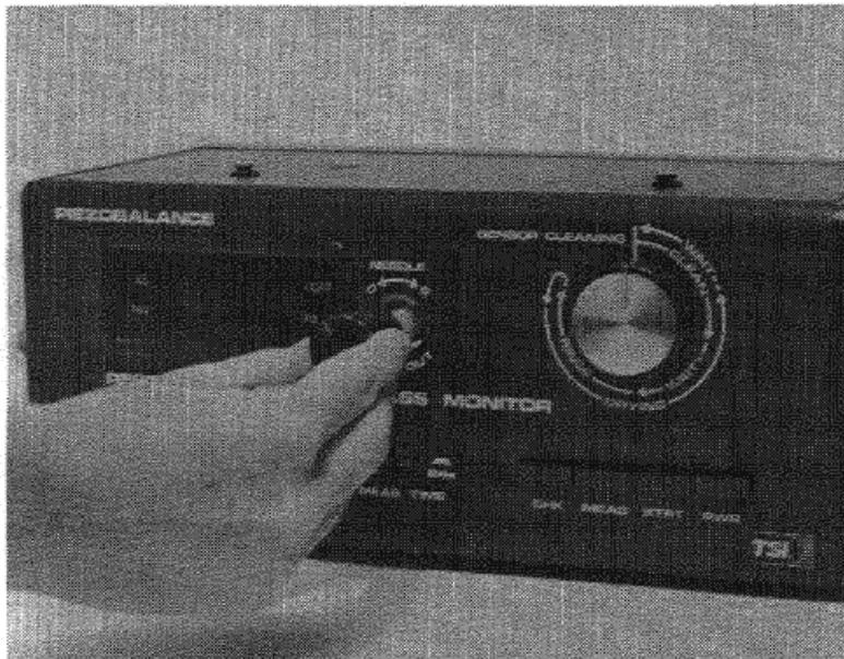
**Figure 32.** Removing the precipitator needle assembly
