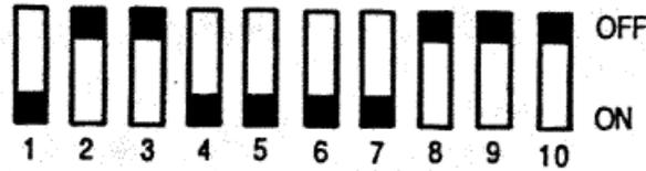
**Figure B-3.** DIP switches set to On and Off at the factory for a setting of 0.00278 (mg/m<sup>3</sup>)/Hz setting.
