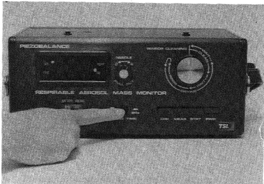
Figure 14. Selecting the Measurement Time
