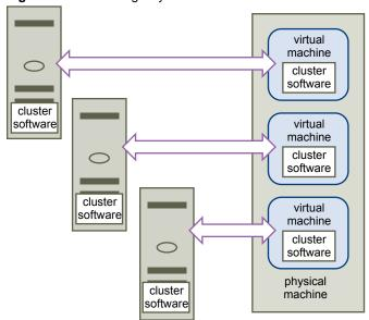
Figure 1-4. Clustering Physical and Virtual Machines
