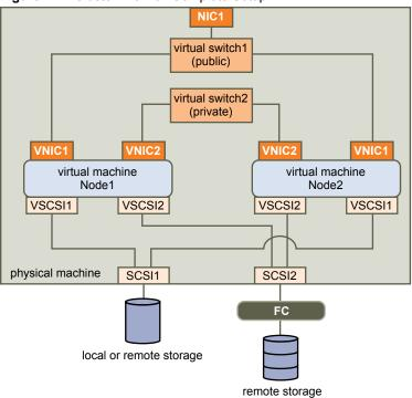
Figure 2-2. Cluster in a Box Complete Setup
