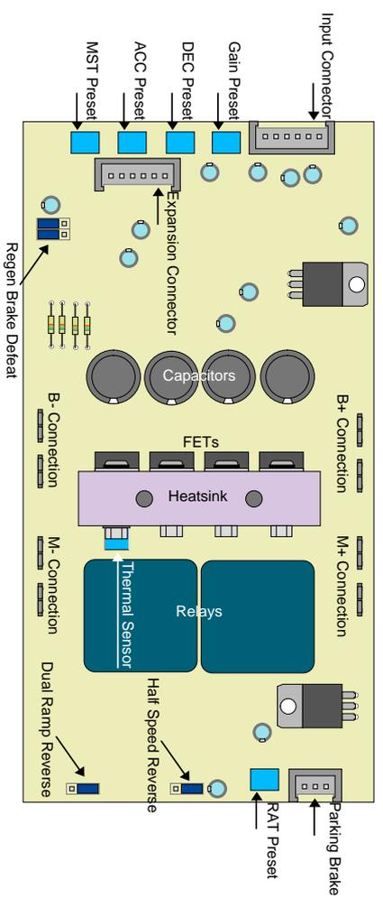
The diagram above shows the Vortex-75 which has four MOSFETs and capacitors. The Vortex-40 has two only. Otherwise, the Vortex-40 is largely the same as the Vortex-75.
