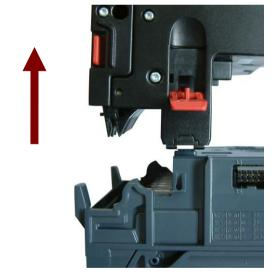
3. To refit the Note Float module, reverse the procedure – make sure that the electrical connectors and latches are lined up correctly
