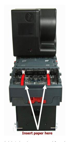
Repeat this procedure until all dust and debris has been removed from both belts. Finally, use a DRY lint free cloth to remove any excess moisture and refit the bezel. The bezel is refitted by pushing the bezel back onto the locating pins and sliding backwards until all six pins are engaged in the slots. The locking arms will then spring back and locate into the bezel.
