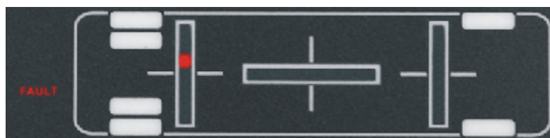
2. Short circuit in rear left Travel valve
