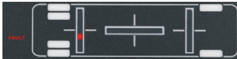
4. Short circuit in rear right Raise valve
