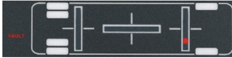
3. Short circuit in front right Lower valve
