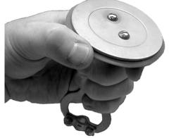
6) After the cup is partially formed, place the plunger assembly into the meter body and press into the piston cylinder.
