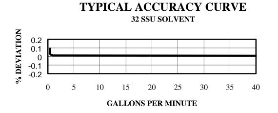
The 682 meter's linear accuracy (percent of error over or under the zero - error level) remains within design parameters (+/- 0.2%) over its 0.2 to 40 GPM flow range. This exceeds the maintenance requirements for accurate custody transfer of product, as specified in the National Institute of Standards and Technology (NIST) Handbook 44.
