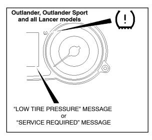
Vehicles equipped with TPMS have a warning light in the instrument panel to notify drivers when low air pressure or a system fault is detected.
