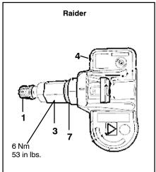
1. Valve stem cap - Valve stem caps designed for TPMS use an internal o-ring to increase sealing, reduce air loss, and prevent moisture and dirt from contaminating the sensor.
