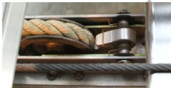
Figure 7. AAD Cam engaging with rope.
