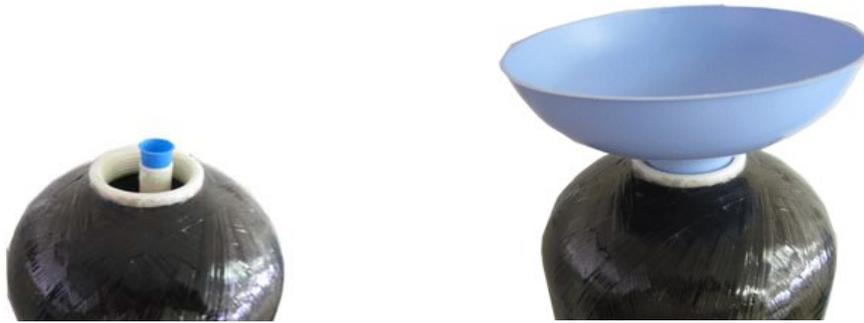
2. Add the filter gravel that came with your system. You want the gravel to cover the bottom distributor screen before adding the Pro-OX media. **Note: Be sure not to let any parts of the bag or other foreign materials enter the tank when you are adding media.**
