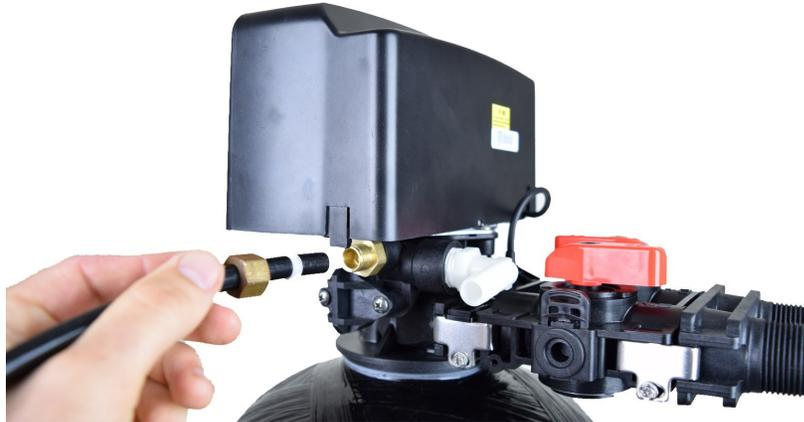
15. Insert 3/8" diameter tubing into the chlorine side tank connection. Screw the nut with the sleeve and Ferrell attached to prevent leaking.
