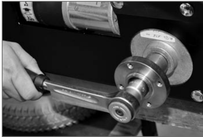
Fig. 21 Loosening the wheel flange screw
