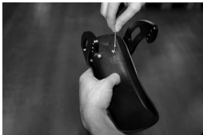
Fig. 26 Mounting the splash guard for caster forks
