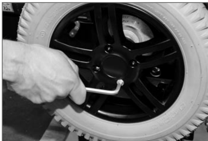
Fig. 20 Disassembling the drive wheel
