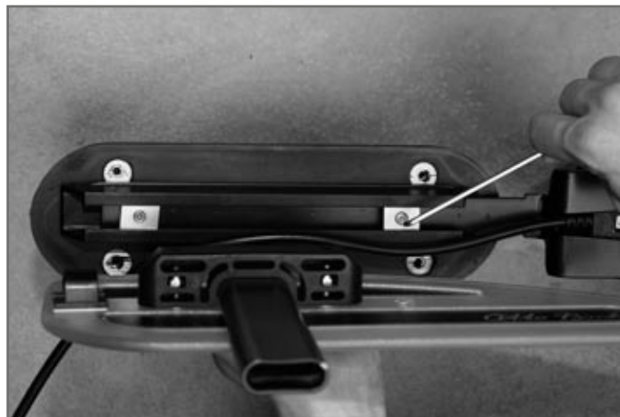
Fig. 29 Replacing the control panel holder
