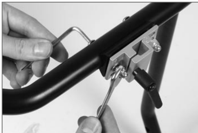
Fig. 50 Assembling the holding device for headrest attachment
