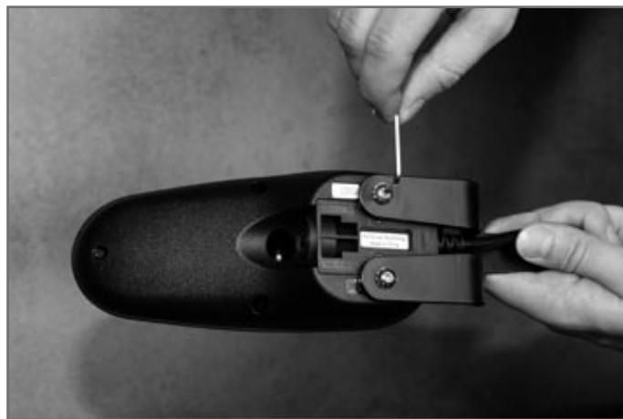
Fig. 27 Replacing the control panel
