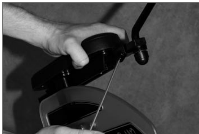
Fig. 48 Retrofitting a rearview mirror
