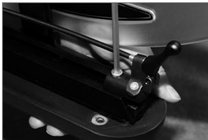
Fig. 46 Attaching the Bowden cable
