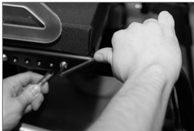
Fig. 15 Adapting the footrest to the thigh length
