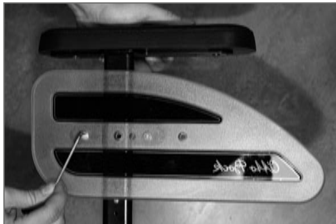
Fig. 12 Replacing the clothing protector
