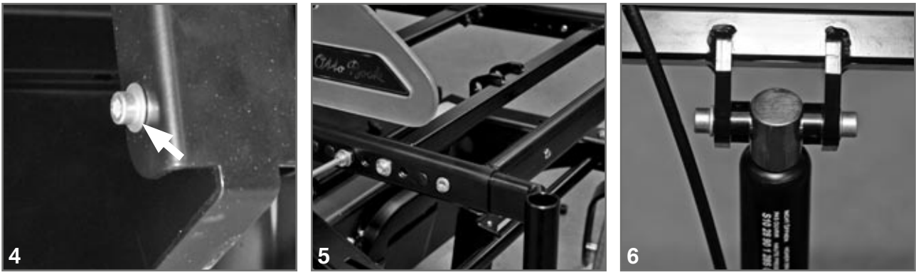
Fig. 45 Retrofitting the mechanical seat tilt mechanism
