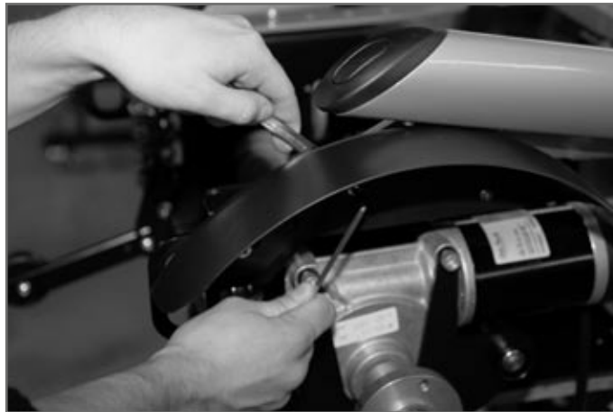
Fig. 23 Mounting splash guards for drive wheels
