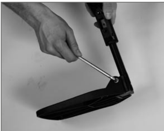
Fig. 18 Replacing the footplate
