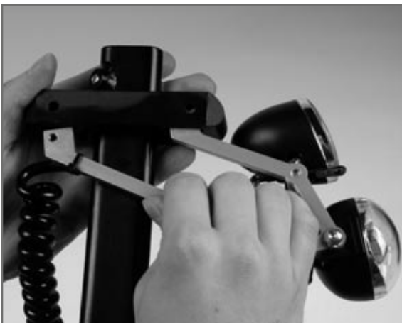
Fig. 32 Retrofitting front lights
