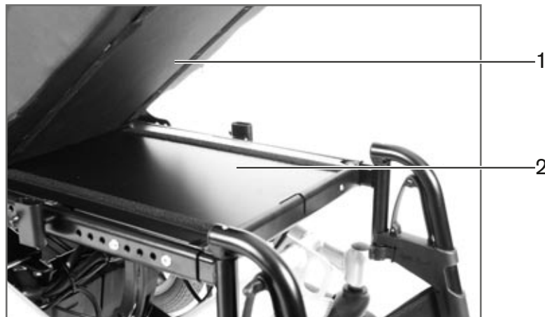
Fig. 40 Replacing the seat plate of the standard seat
