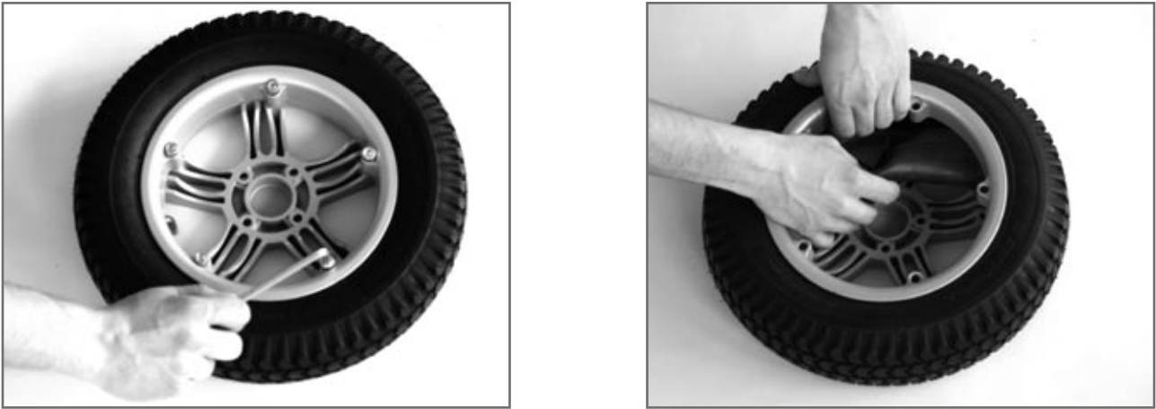
Fig. 19 Removing the casing
