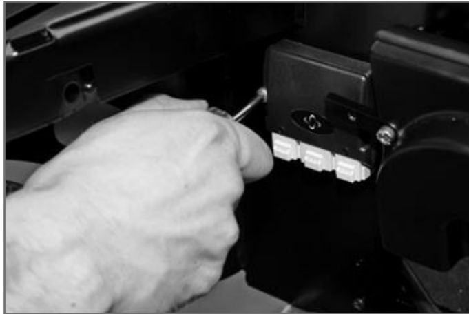
Fig. 30 Mounting the light module
