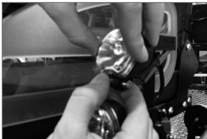
Fig. 34 Replacing the halogen lamp of a front light
