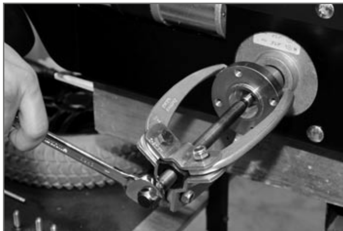
Fig. 21 Loosening the wheel flange screw
