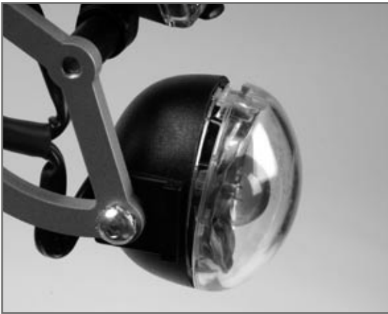
Fig. 35 Replacing the front direction indicator
