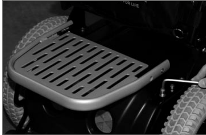
Fig. 52 Mounting a luggage carrier
