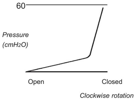
As shown in the graph above, further clockwise rotation causes a rapid increase in opening pressure so that in the fully closed position, the valve functions as a 60 cmH<sub>2</sub>O excess pressure relief valve.
