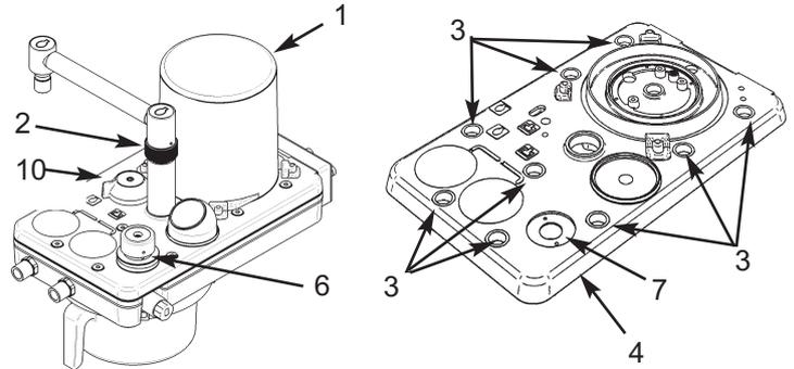
4. Invert the bellows plate assembly and remove the two screws (6) and washers.
