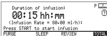
1. Press the Command wheel to **CONFIRM** the infusion mode.
