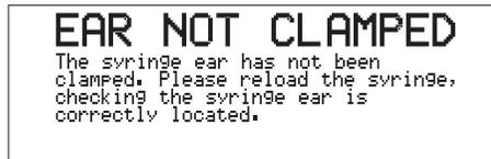
After three seconds this screen is replaced and the message line displays a short warning message:
