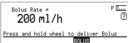
2. Change the bolus rate using either the Command wheel or numeric keypad.
