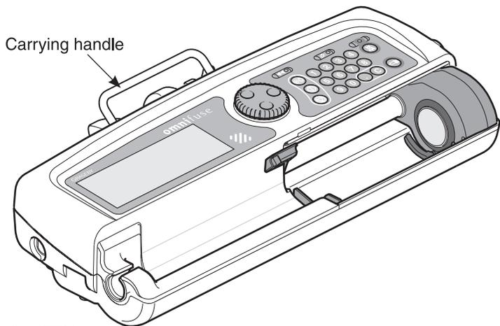
**CAUTION: Never carry the pump except by the handle. Failure to do so may result in damage to the case, or you may drop the pump and cause it internal damage.**
