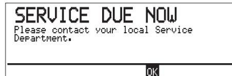
The pump can still be used. To continue with your setup, simply press the Command wheel. If however you wish the pump to be serviced, switch off.
