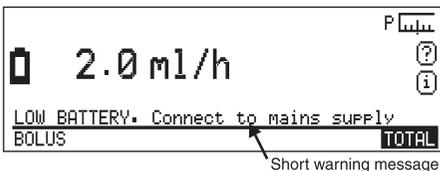
The message is repeated until you connect the pump to an AC mains power supply, or end the infusion and switch off.
