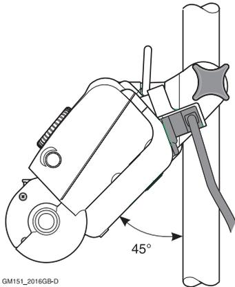
This angle makes it easy for you to read the screen and also gives you good access to the keypad and Command wheel. To clamp the pump to an IV pole:
