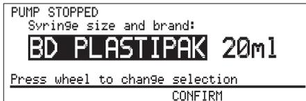
The pump can sense the *size* of syringe you have loaded, but it cannot sense the *brand*.
