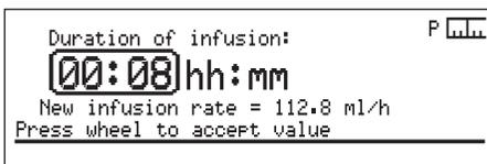
2. Turn the Command wheel, or use the numeric keypad to set the number of hours and minutes you want the infusion to run, from now. Press the Command wheel to accept the value.
