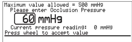
Turn the Command wheel or use the numeric keypad to alter the alarm setting, then press the Command wheel to exit the display.
