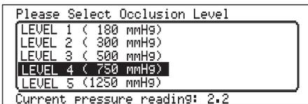
3. Turn the Command wheel to highlight the new level at which you want the occlusion level alarm to sound.
