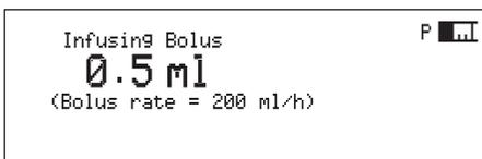
3. Press and hold down the Command wheel to deliver the bolus. When the dose is complete, release the Command wheel.
