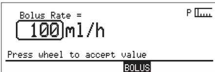
1. If the bolus rate displayed is not applicable, turn the Command wheel to highlight the bolus rate, then press the Command wheel.
