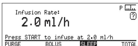
1. The **WAKE ME** hotspot is already highlighted. Press the Command wheel to wake the pump and exit from Sleep mode.
