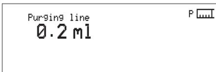
**WARNING:** To avoid patient embolism, ensure that the patient tubing is purged of all air bubbles before administering any medication. The pump provides a purge facility to assist with this process. The presence of air within the medication can result in complications leading to patient injury or death.
