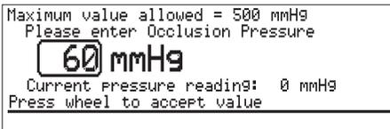
You will see a screen like this, showing the occlusion pressure alarm limit, the current alarm setting (boxed) and pressure reading.
