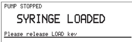
1. Ensure that the line to the patient is clamped, or disconnected. Switch on the pump if it is switched off. Lift up the barrel clamp if it is closed - you will see this message
