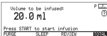
1. Press the Command wheel to **CONFIRM** the infusion mode. See page 4 - 7 if the pump displays a different infusion mode and you need to change to Preset Volume.
