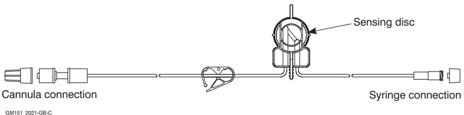
The set is suitable for use with a syringe of 5 ml capacity or larger. Always prime and connect the line according to the instructions for use on the Flo- Safer™ instruction leaflet.
