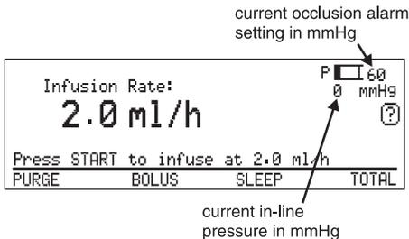
The In-line Occlusion Pressure icon shows how close the pressure is to the alarm level:
