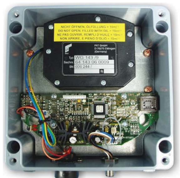
CAN-Bus electronics in angle sensor box.
