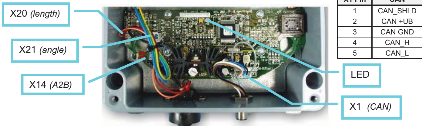
CAN-Bus electronics in angle sensor box.
