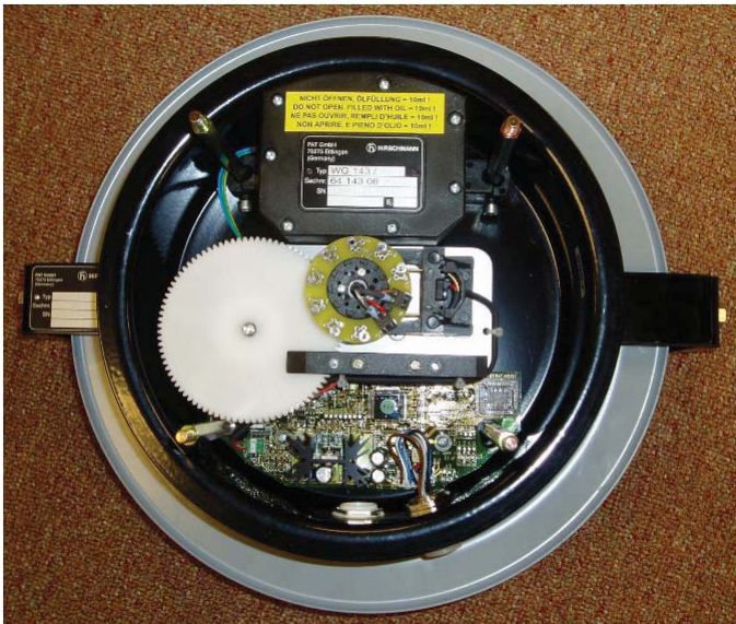
CAN-Bus electronics in cable reel.
