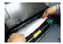
3. If the paper is not present, check if the Fuser Exit and Reverse actuator's return action as the EDC Mode just checks on/off. If so, check the actuator springs of the Fuser Exit and Reverse return spring tension is sufficient,. and sensor arm works smoothly. (EDC Mode -> Test Routines -> Engine Diagnostic Test -> 102-370 / 102-xxx)
