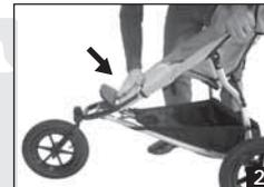
Place pressure on heel rest to ensure sliding locks are fully engaged.
