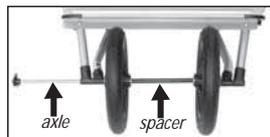
INSERT AXLE. Also insert spacer between front wheels.
