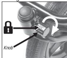
**TO LOCK:** Turn knob so locked symbol is at the top. Then swivel wheel under stroller until it locks into place.
