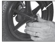
De-press quick release clip and slide wheel off axle.
