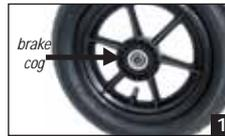
Check that brake cog is on the inside next to stroller frame.
