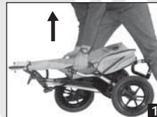
Grip stroller near sunhood joints, and lift.
