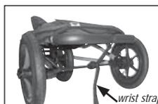
Wrist strap can be used to hold stroller together in its fully folded position. Loop wrist strap around rear axle then fasten.
