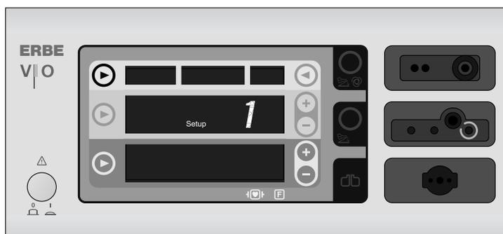
1. When switching on the unit, press and hold the top left selection button. The unit switches to the Setup.
