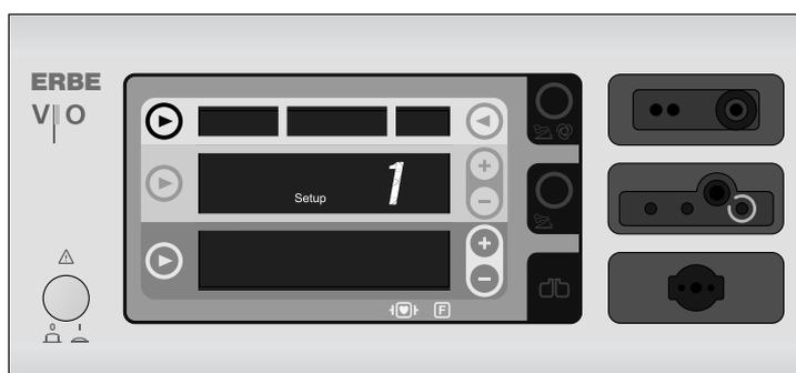
1. When switching on the unit, press and hold the top left selection button. The unit switches on to the Setup and shows <Setup 1> in the yellow display. The yellow Plus/Minus buttons can be used to switch between setup settings. For more about setup settings, see table on page 13.
