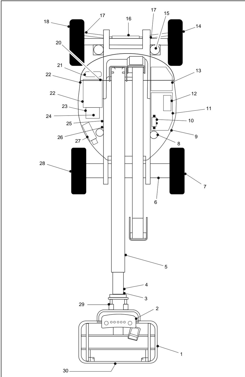
**Figure 2-3. Daily walk-around Inspection. (Sheet 1 of 3)**
