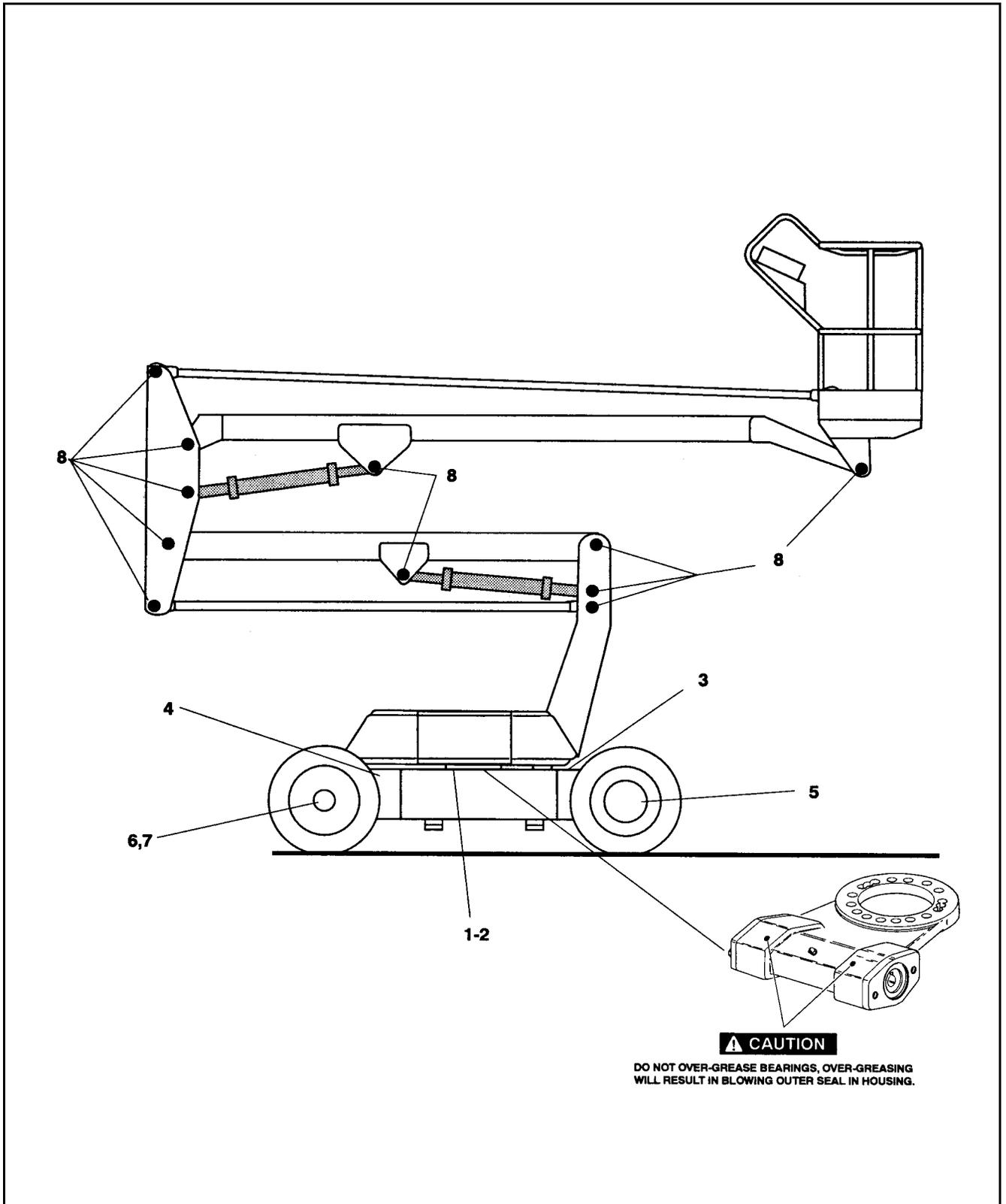
Figure 2-4. Lubrication Chart - 30 electric. (Sheet 1 of 6)
