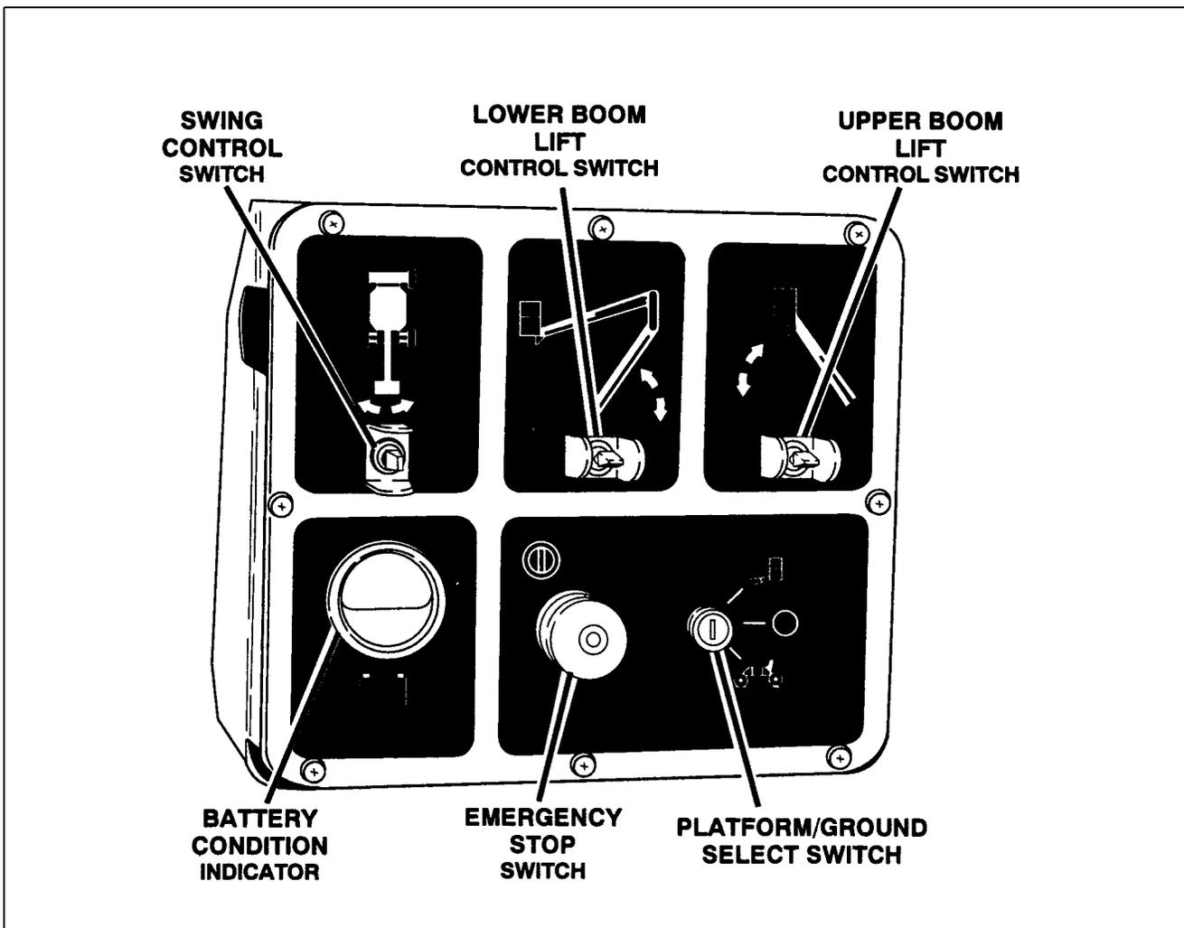
Figure 3-3. Ground Control Station, 30 electric. (Sheet 1 Of 4)
