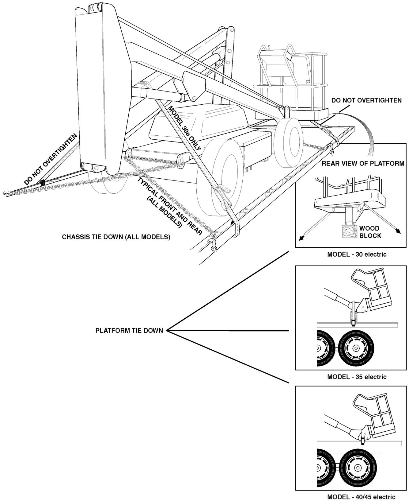
Figure 4-3. Chassis & Platform Tie Down. (All Models)
