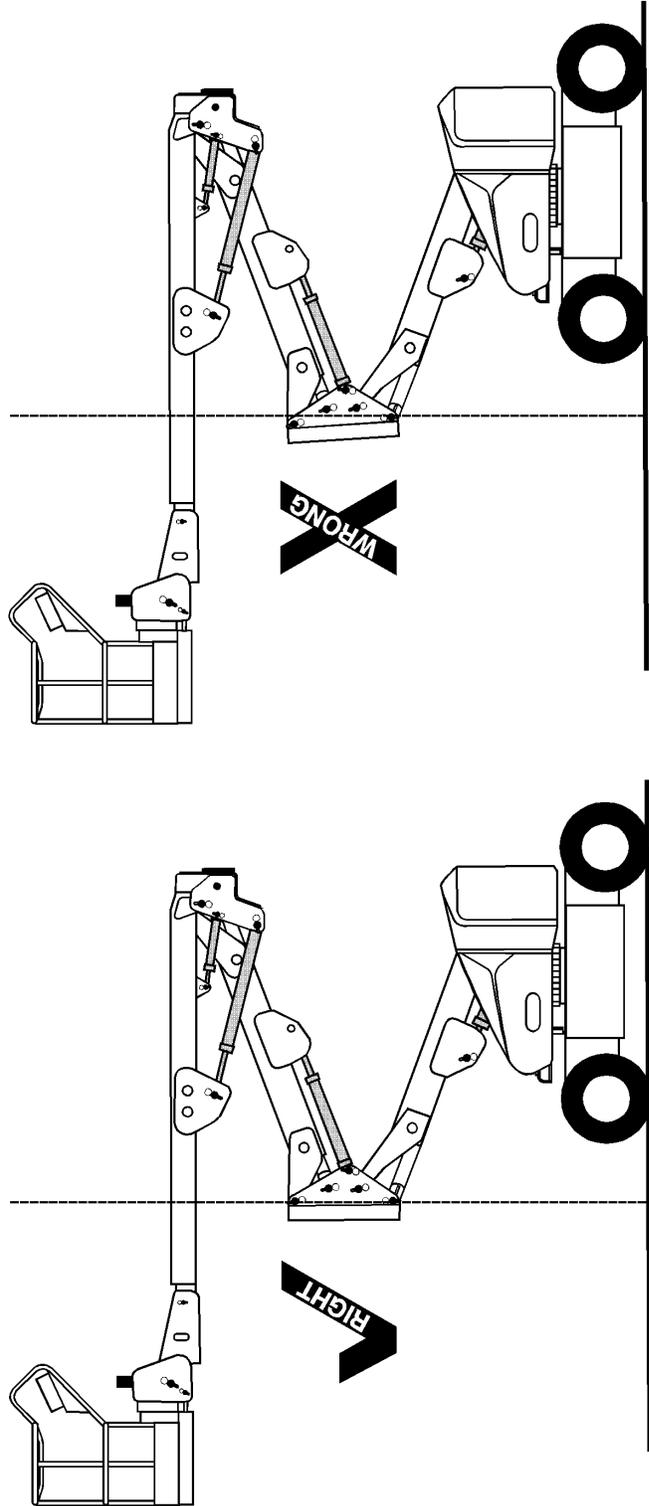
Figure 4-2. Upright Positioning Models 40e and 45e.
