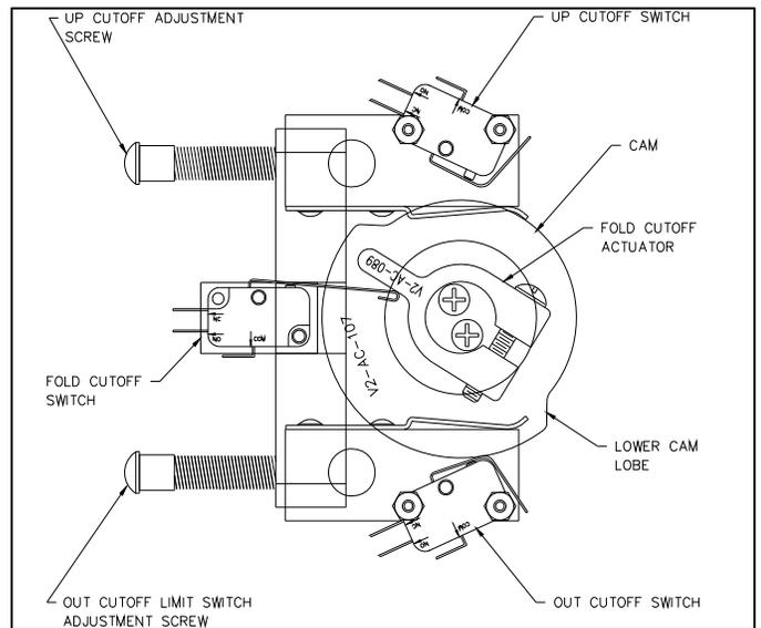
**FIGURE 2-17: LIMIT SWITCH ADJUSTMENT DIAGRAM**
