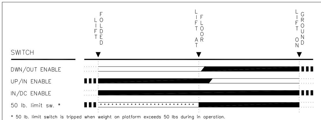
FIGURE 3-6: LIMIT SWITCH ACTUATION DIAGRAM
