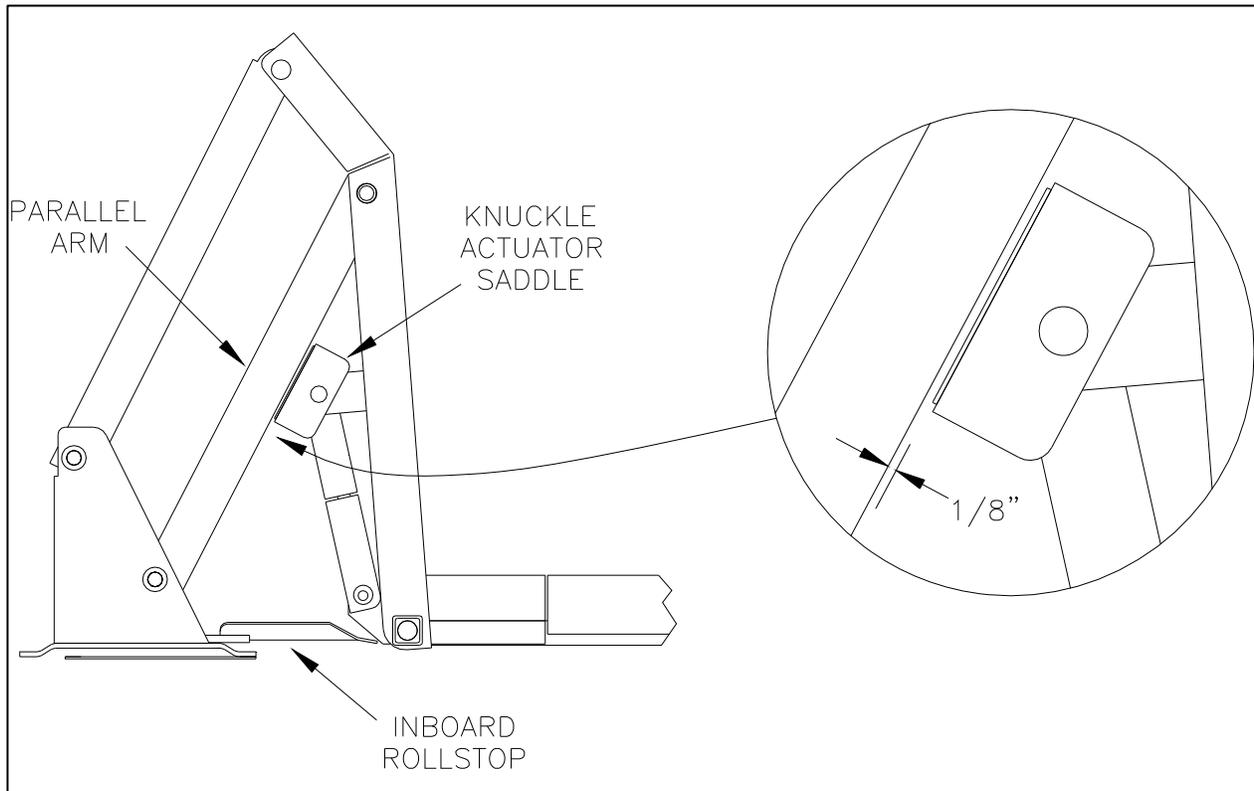
**FIGURE 2-18: LIMIT SWITCH ADJUSTMENT CLEARANCE**
