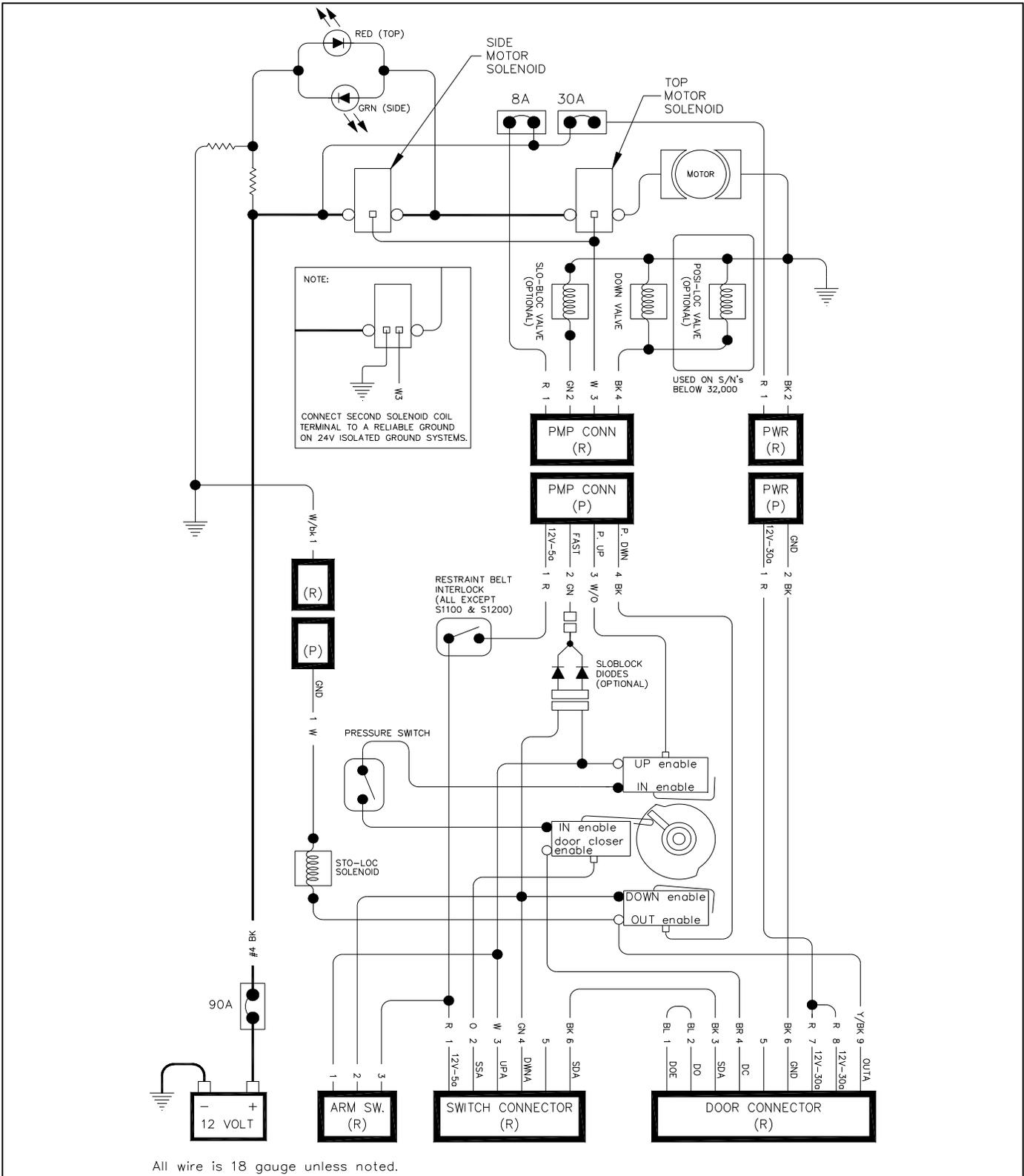
FIGURE 3-7: WIRING DIAGRAM FOR LIFT W/DOOR OPERATOR
