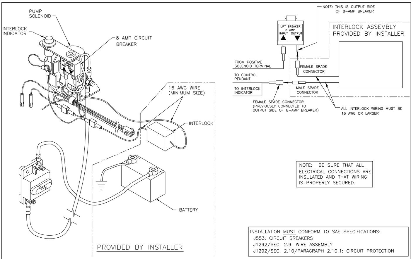
**FIGURE 2-14: INTERLOCK METHOD #1 DIAGRAM**
