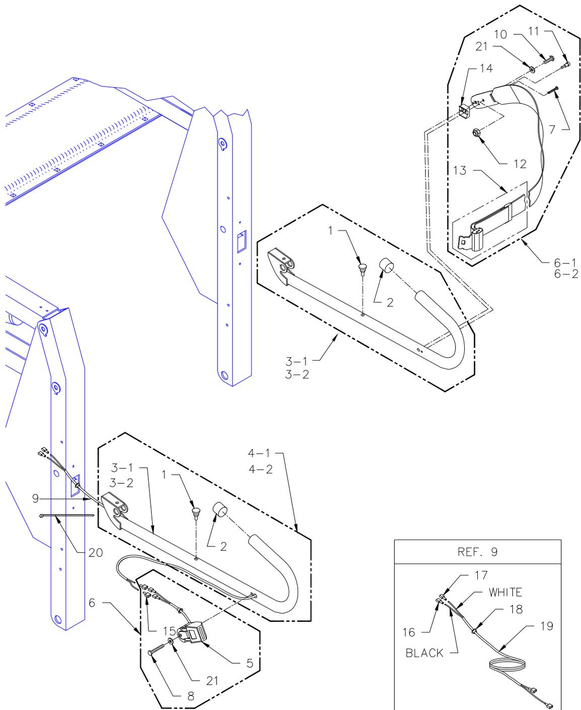
FIGURE 4-9: K-2005 (ADA) HANDRAIL ASSEMBLY
