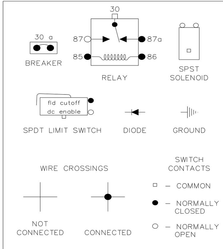
FIGURE 3-5: ELECTRICAL WIRING DIAGRAM SYMBOLS
