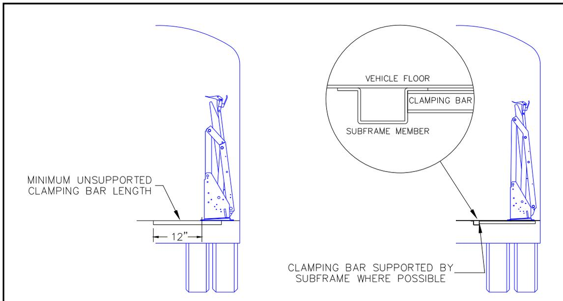
**FIGURE 2-7· BUS CLAMPING BAR ARRANGEMENT**
