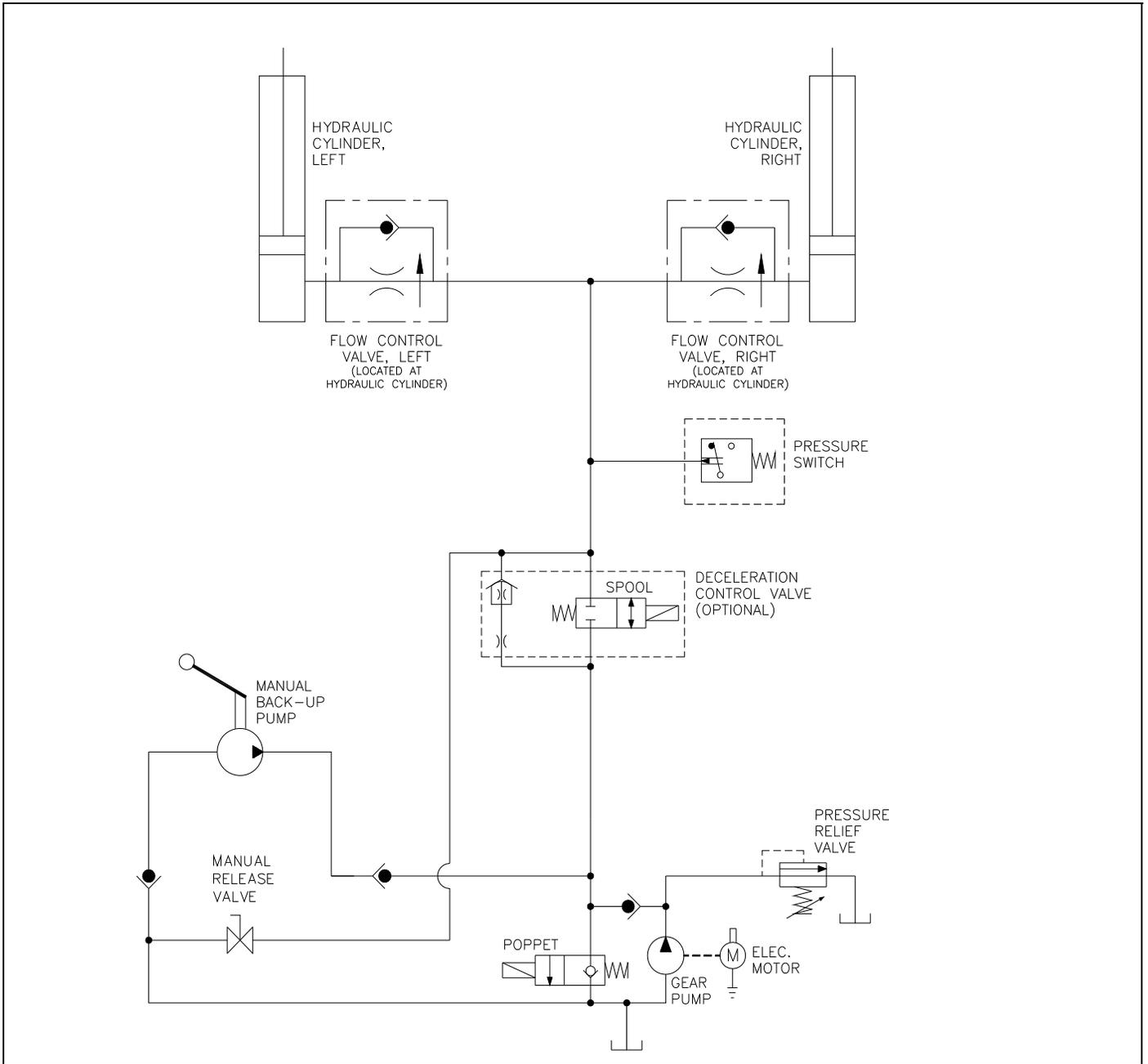
**FIGURE 3-2: K-SERIES HYDRAULIC CIRCUIT DIAGRAM**
