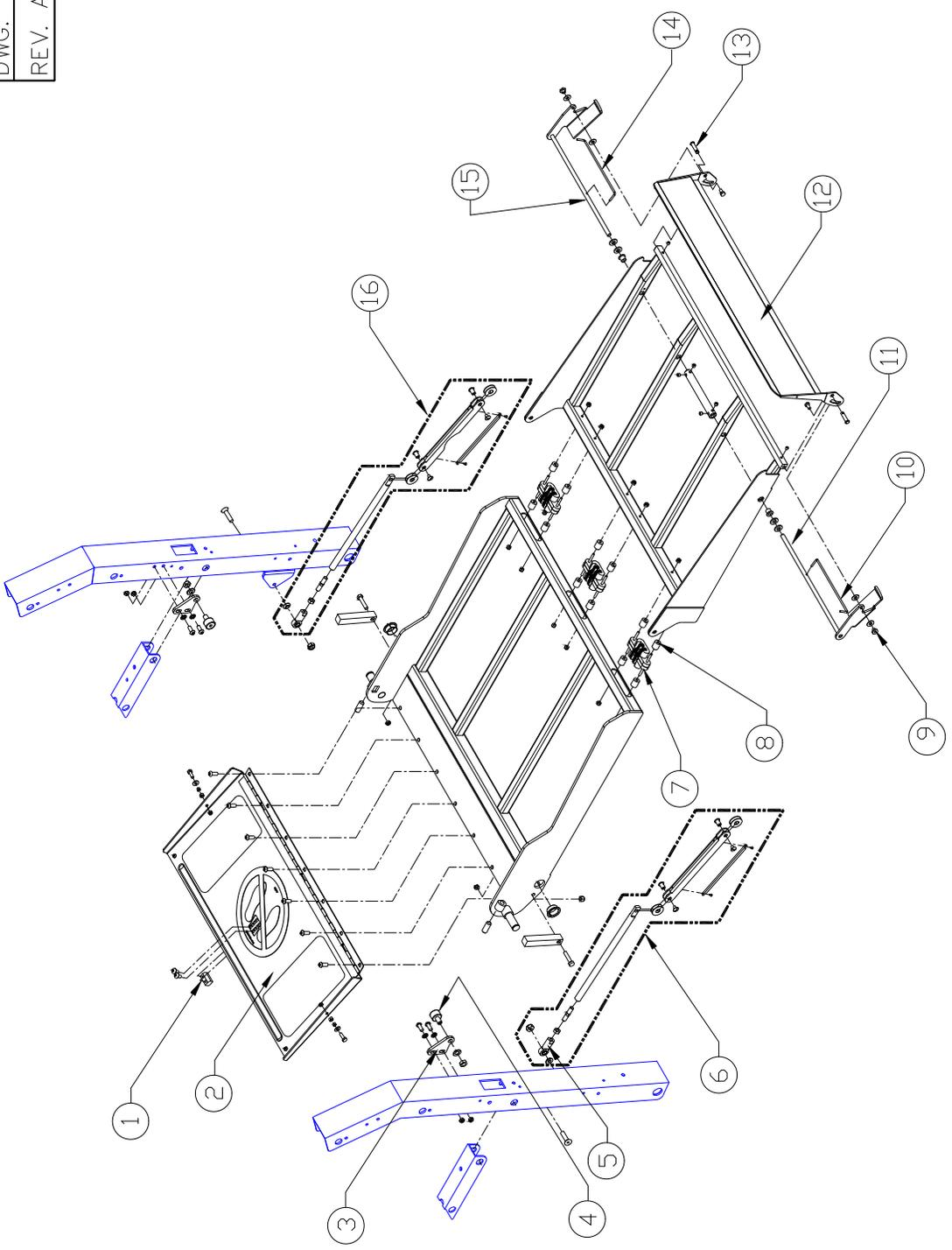
**FIGURE 4-6: K-LIFT FOLDING PLATFORM ASSEMBLY, 2003 & 2005**
