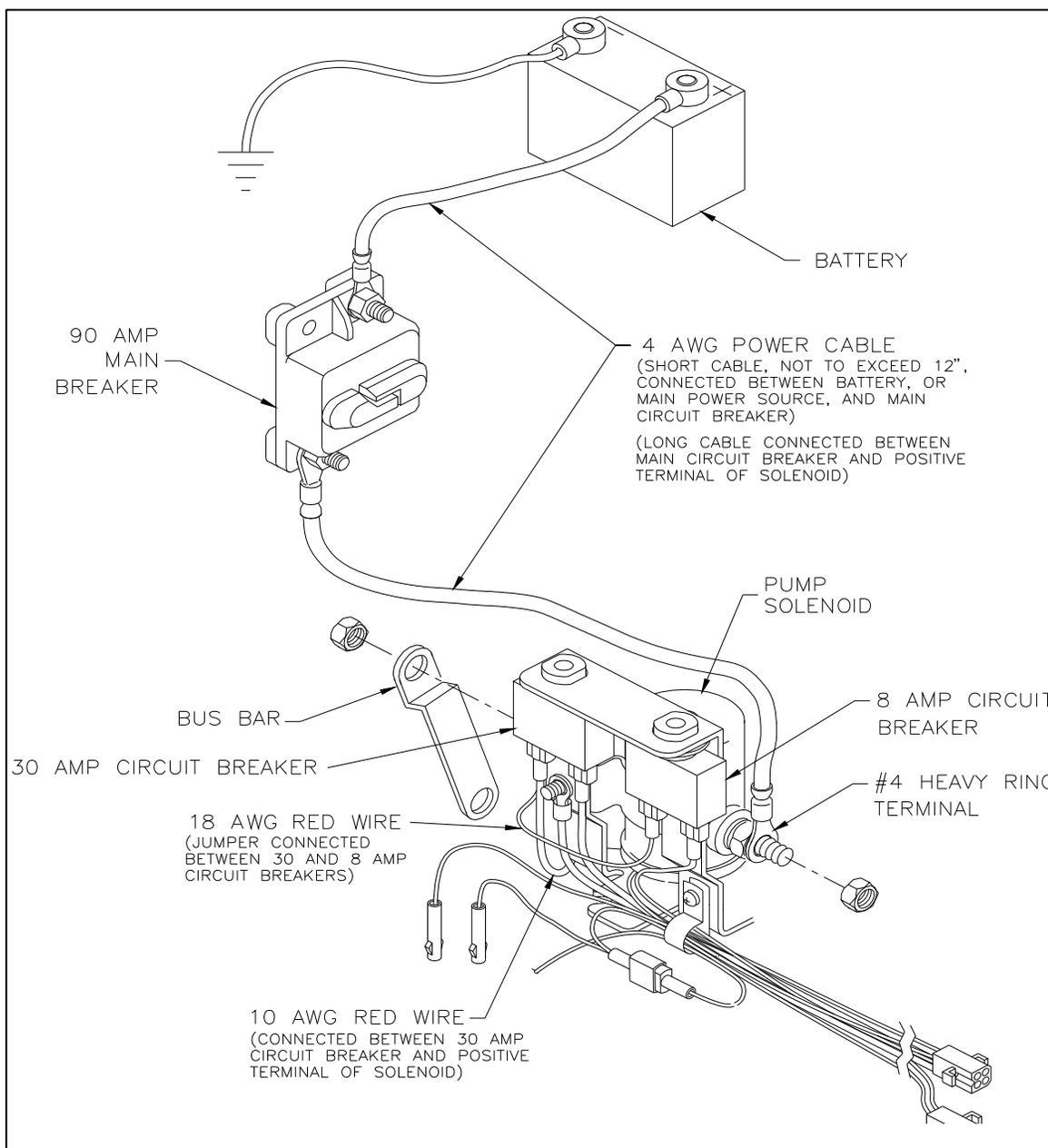
FIGURE 2-9- ELECTRICAL INSTALLATION DIAGRAM
