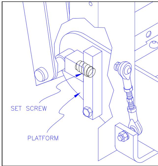
**FIGURE 2-19: PLATFORM SET SCREWS**
