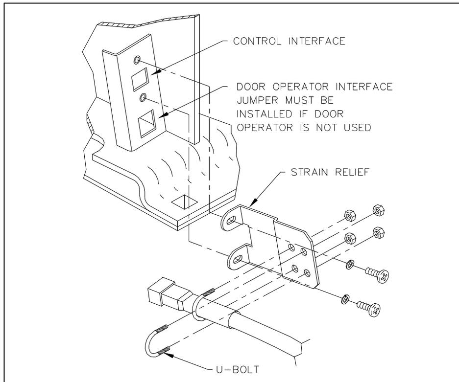
*FIGURE 2-12. CONTROL INTERFACE AND STRAIN RELIEF*
