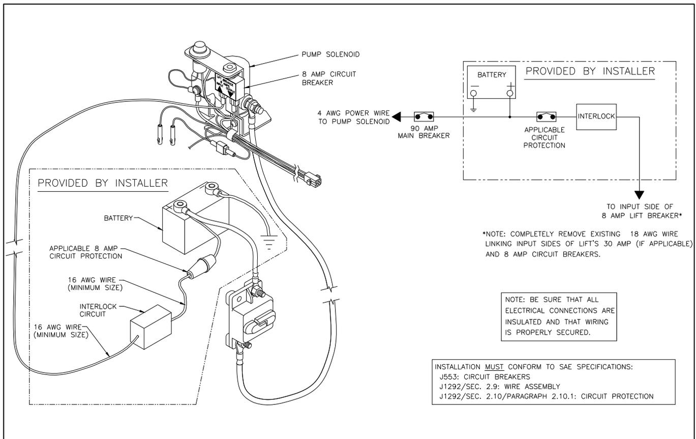
**FIGURE 2-15: INTERLOCK METHOD #2 DIAGRAM**
