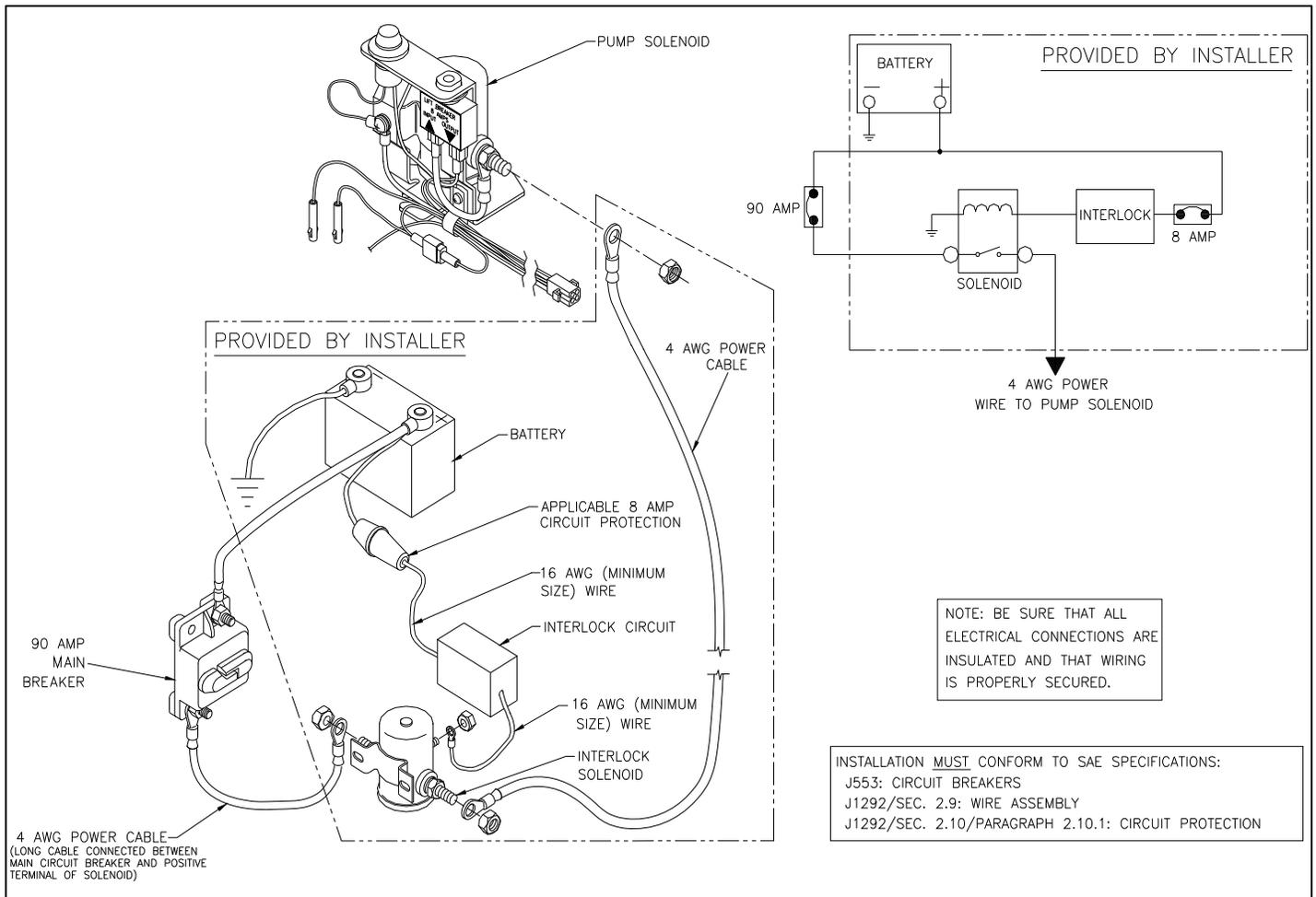
**FIGURE 2-16: INTERLOCK METHOD #3 DIAGRAM**
