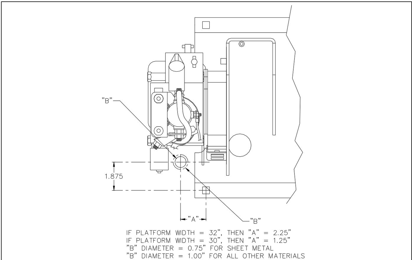
**FIGURE 2-10. POWER CABLE ACCESS HOLE.**
