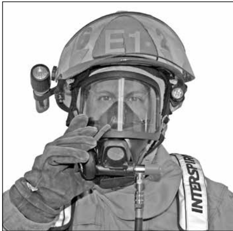
Ambient air hatch open
