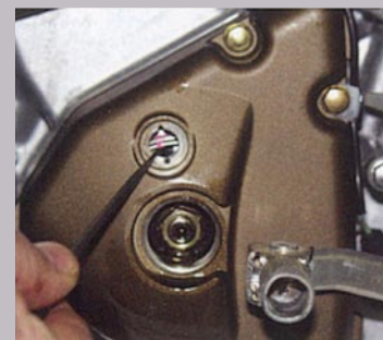
Fig. B: Additionally the dots (A & B) on each camshaft should line up with top surface of cylinder head (C).
