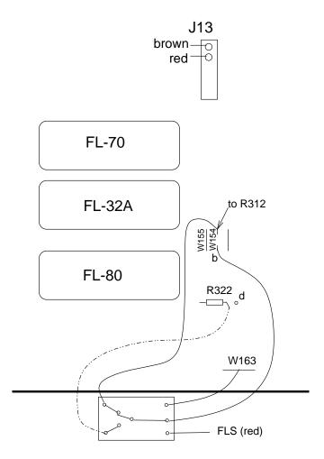
Figure 6: Pictorial of the Filter Modification
