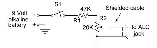
Figure 3: QRP adaptor for IC-765
