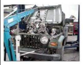
Using an approved engine hoist, lower the engine into the compartment. Pay attention to the exhaust manifolds and the radiator (removing the radiator is a good idea). The engine may not slide fully into the compartment due to firewall interferences (check the clearance on both the driver's and passenger side around the engine heads
