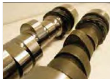
Figure 4 Longer rod engines seem to prefer shorter durations and wider lobe separation.
