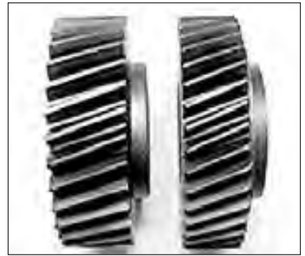
Figure 3 It's easy to confuse the two gears, but putting the wrong driven gear into a Ford engine will cause real problems.
