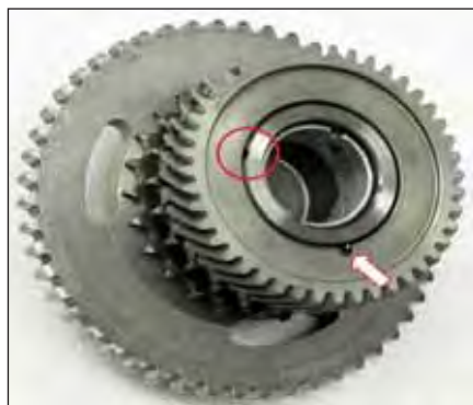
Figure 5 The circle shows where the roll pin (arrow) and spline gear should be aligned for proper timing of the balance shaft on the 3.7L. This assembly has spun on the center shaft over 90 degrees.
