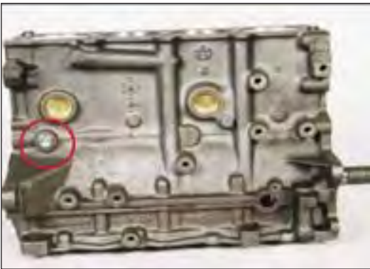
Figure 1 The hole for the oil sender on the passenger side of the 2.4L was moved back about 6" in 2001 so it's much closer to the bell housing
