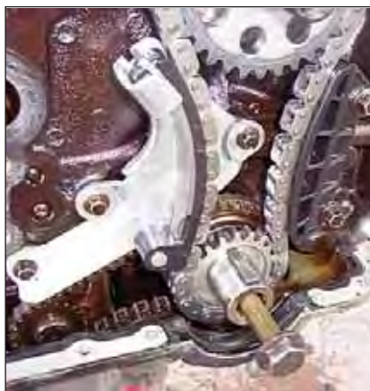
Figure 6 The patented "Offset Y-drive" uses three timing chains, one from the crank to the jackshaft, one in the front of the engine to drive the cam for the left bank and one on the back of the engine to drive the cam for the right bank.
