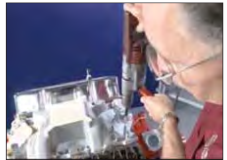
Figure 2 Attach a drill to the end of a priming tool and spin oil pump at a minimum of 500 rpm until oil reaches rockers.
