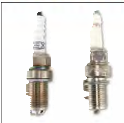
Figure 1 As a rule of thumb, you can expect to require one heat range colder than the factory-supplied plugs for every 75-100 horsepower you've add with your modifications.
