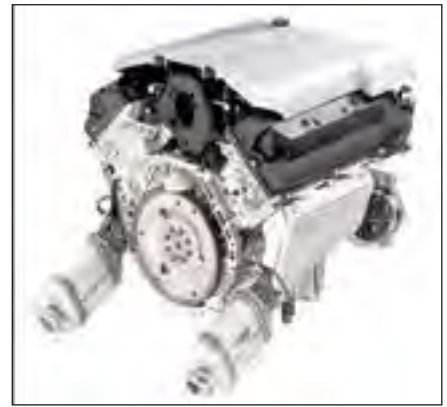
Figure 7 Certain late model General Motors vehicles may be equipped with a new style of catalytic converter, technically known as the close-coupled catalytic converter. Engine failures can damage the converters which, if not inspected properly, can then cause subsequent damage to a replacement engine.
