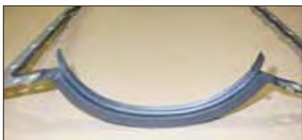
Figure 5 The oil pan was redesigned in 1994 and so was the gasket. The wedge seal is no longer used because its shape is built into the gasket. Silicone is still necessary across the main cap and in the cavities between the cap and the block.
