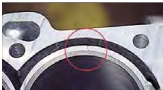
Figure 8 The aluminum 4.6L Cadillac block may crack outside the cast iron cylinder liner and is extremely hard to detect. The above crack became visible only after the deck face was machined.
