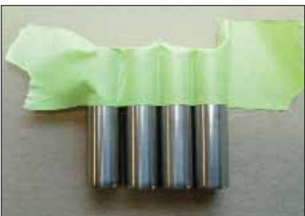
Figure 1 It's often difficult to see when installing guides in OHC heads. Mark with graphite spray for correct depth.
