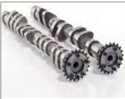
Figure 1 Dimensional differences between the camshaft sprockets and the cam timing chain may create a rattling noise on some Volkswagen 16-valve engines that can be heard from the cylinder head at approximately 2,000 rpm.
