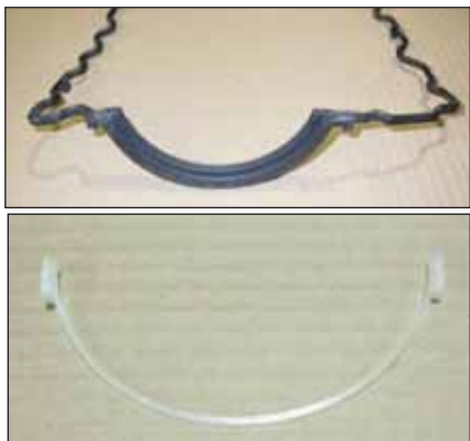
Figure 4 The oil pan gasket for the '90 to '93 4.0L Ford engine (top) will include a plastic wedge seal (bottom) that goes into a groove in the main cap
