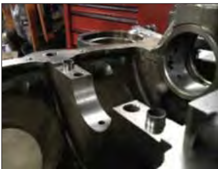
Figure 3 Ream to one half the distance of the dowel, then do the same with the caps. Be sure to sink the holes at least .015" to keep from bottoming the dowels into the cap.
