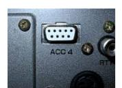
The DB9 connector is fixed without additional screws by clamping it between the rear panel and the metal supports. Proceed as follows:
