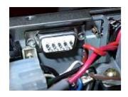
Connect the DB9-pins to the relay outputs of the band decoder using flat ribbon cable. Ground connection is made via the metal case of the DB9 connector. Remember to connect the case of the DB9-plug to ground.
