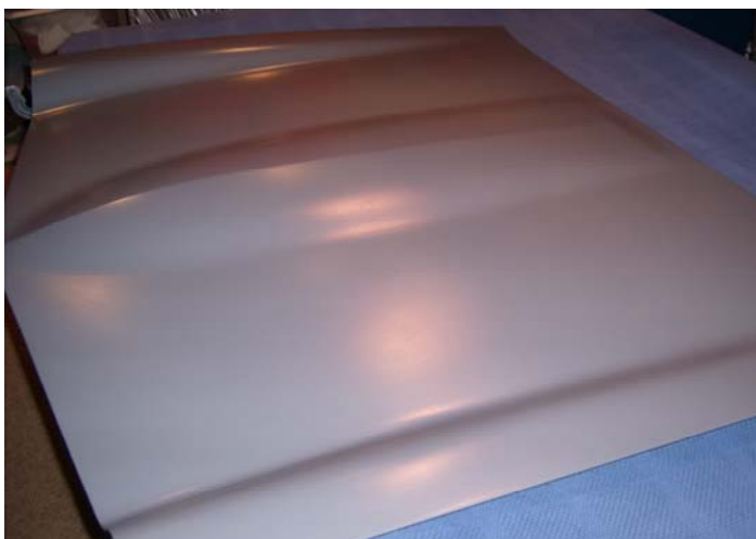
Top of the hood after two medium-dry coats of epoxy primer.
