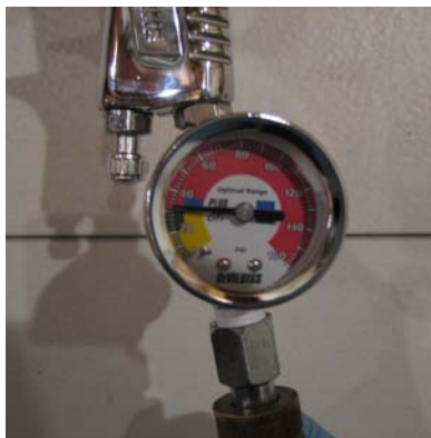
Mount a pressure gauge and regulator at the gun air inlet for the most accurate reading.
