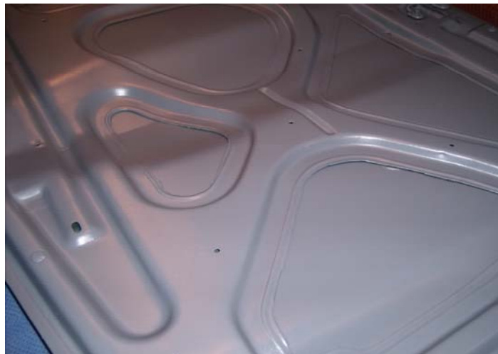
Back of the hood nice and smooth after removal of the old rust proofing, sanding and application of epoxy primer.
