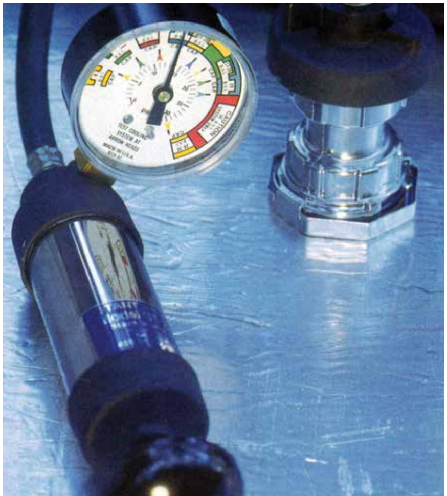
If your pressure tester doesn't have the correct adapter, you can acquire the Nissan special service tool J-33984-A.
