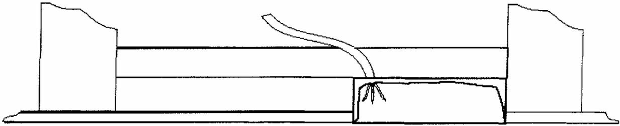
Secure the top portion of the lamp to the ceiling with the two 8-32 threaded rods provided – as shown in diagram.
