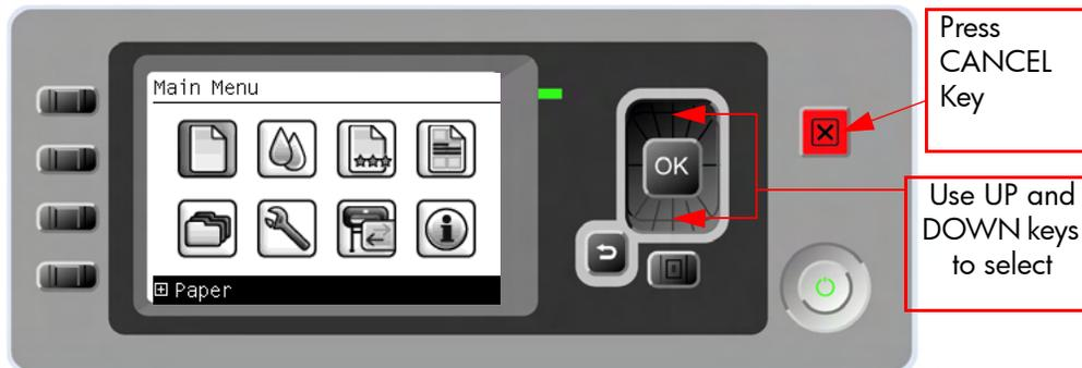
3. Use the **Arrow** keys to scroll to the **Service calibrations** menu option and press the **OK** key.
