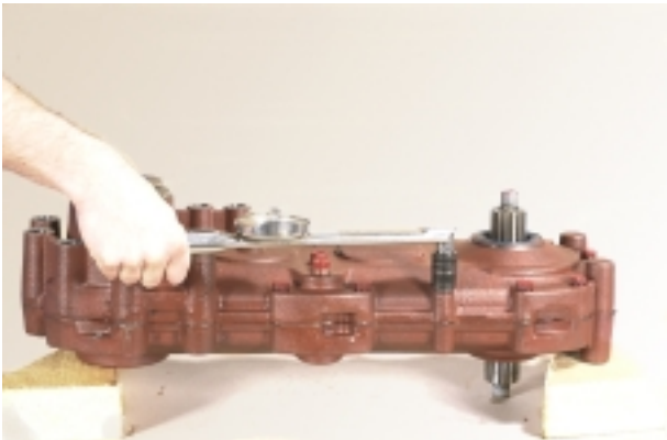
Figure 46 Tighten screws to specified torque. (See torque chart).
