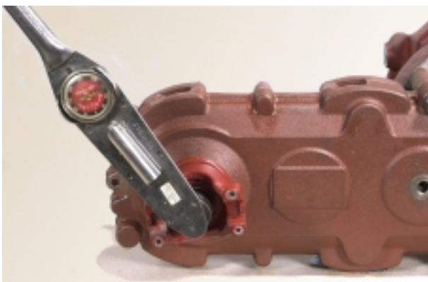
Figure 62 Block flanges to prevent turning. Tighten flange nuts to specified torque. See assembly instructions page 7-4.
