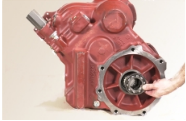
Figure 51 Install output shaft rear bearing in case against locating ring.
