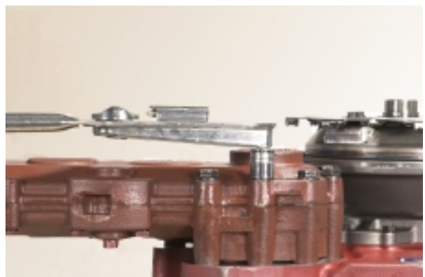
Figure 59 Install drop box mounting screws and lockwashers. Tighten to specified torque. (See torque chart).
