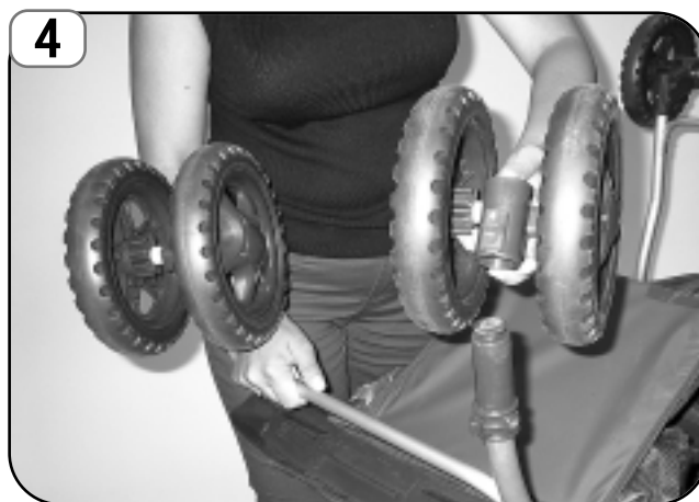
Position each front wheel assembly onto each of the front legs. Pull back on tab, slide into position and release tab. IMPORTANT! Pull firmly on all wheel assemblies to be sure that they are securely attached.
