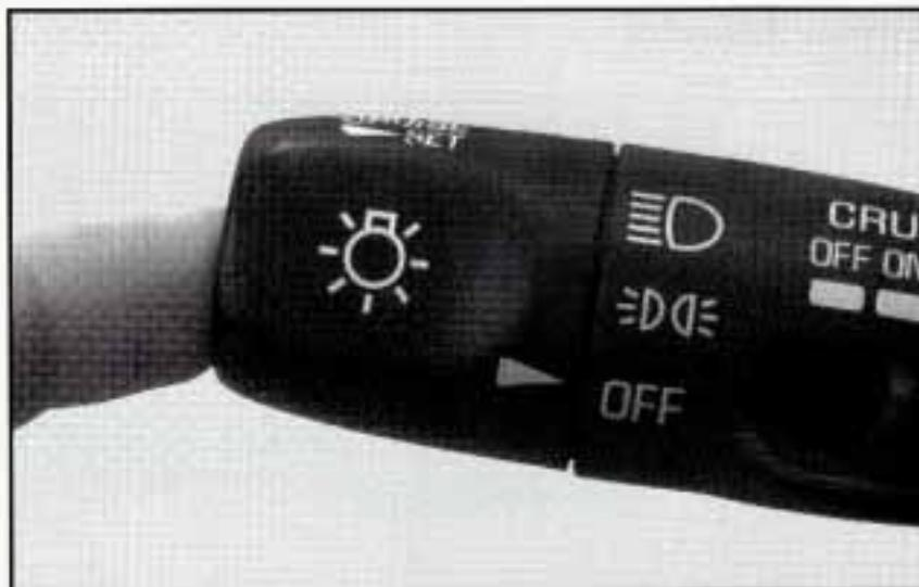
3. Push the CRUISE SET button at the end of the lever and release it. The cruise set speed will be displayed by the Driver Information Center (DIC).
