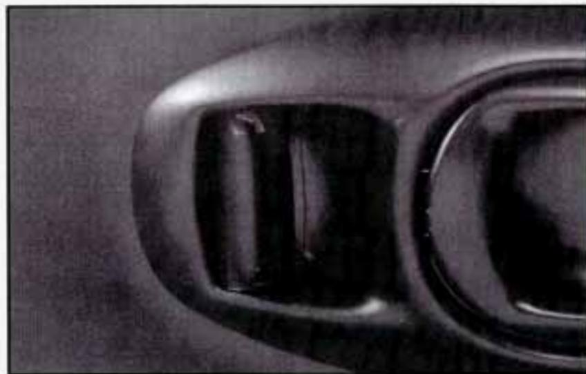
From the inside: To lock the door, move the lock control on the door forward. To unlock it, move the lock control on the door backward.
