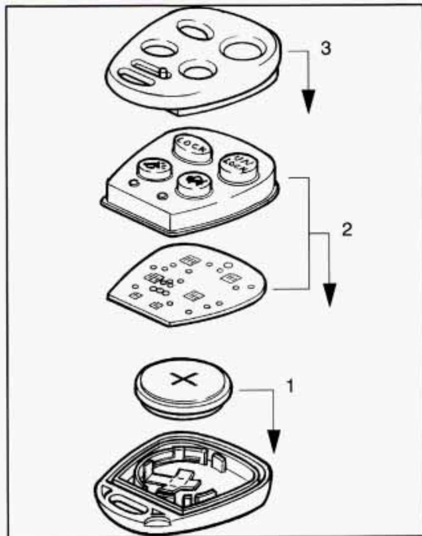
1. Insert a coin into the slot on the back of the transmitter and gently pry apart the front and back.
