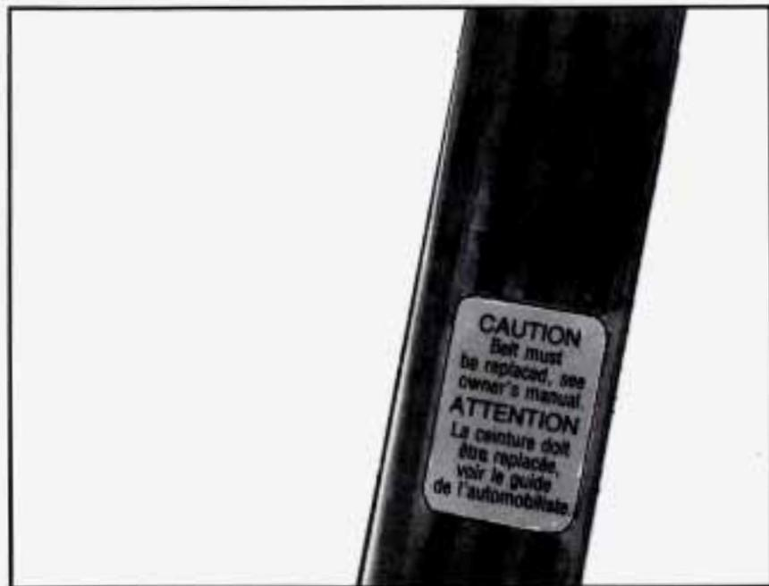
If you ever see a label on the driver's or passenger's safety belt that says to replace the belt, be sure to do so. Then the new belt will be there to help protect you in a collision. You would see this label on the belt near the latch plate.
