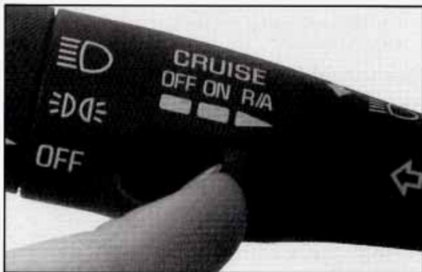
Once you're going about 25 mph (40 km/h) or more, you can move the cruise control switch to R/A (Resume/Accelerate) for about half a second. The DIC will display the cruise set speed.
