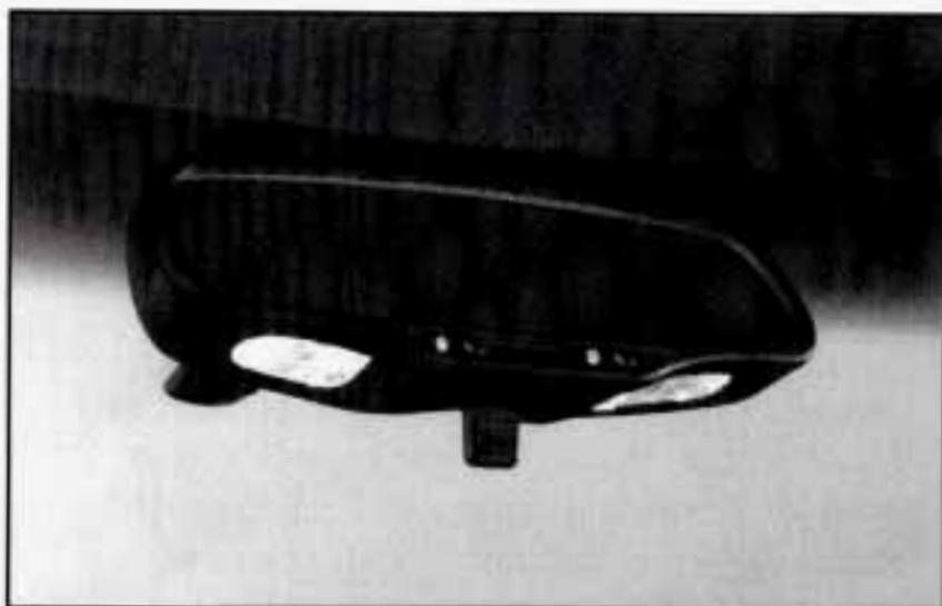
Your inside rearview mirror includes two reading lamps. The lamps will go on when a door is opened. When the doors are closed and the ignition is on, each lamp can be turned on individually by moving the switch (each lamp has its own switch) to ON.
