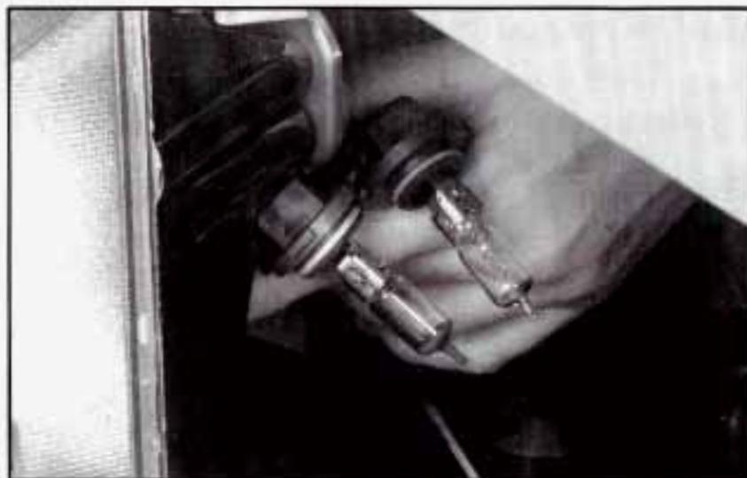
6. Reach behind the lamp and turn the bulb to the left to remove it. Don't touch the halogen bulbs. The inner bulb is the high beam and the outer bulb is the low beam.
