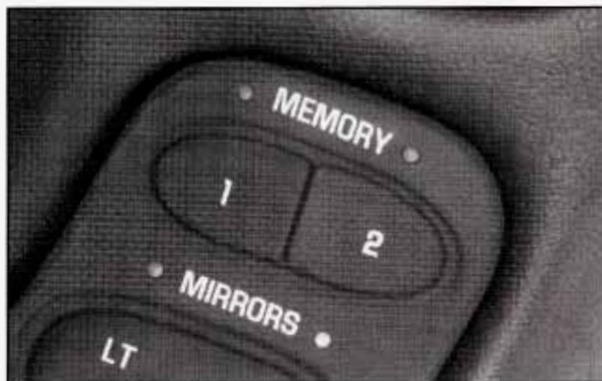
MEMORY can store and recall the vehicle settings for the driver's seat position, the outside rearview mirror position, comfort control temperature, fan speed and mode settings, radio presets, tone, volume, playback mode (AM/FM, tape or CD), last displayed station, compact disc position and audio tape direction.
