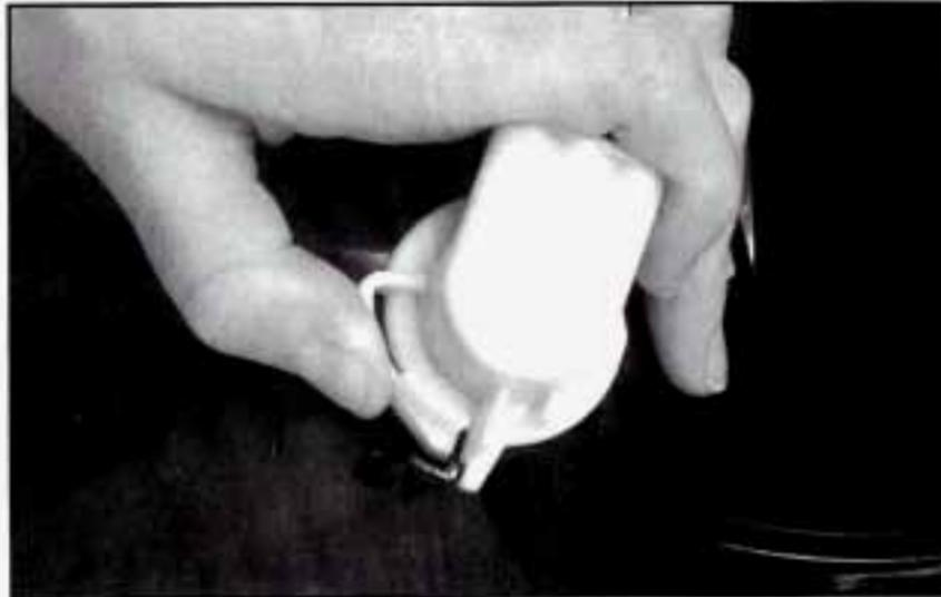
3. To remove the socket with the bulb, squeeze the tab while you turn the socket to the left.
