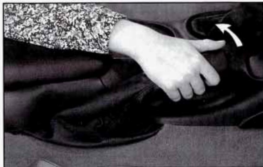
To set the parking brake, hold the brake pedal down. Pull the parking brake lever. This sets your parking brake. If the ignition is on, the brake system warning light will come on.
