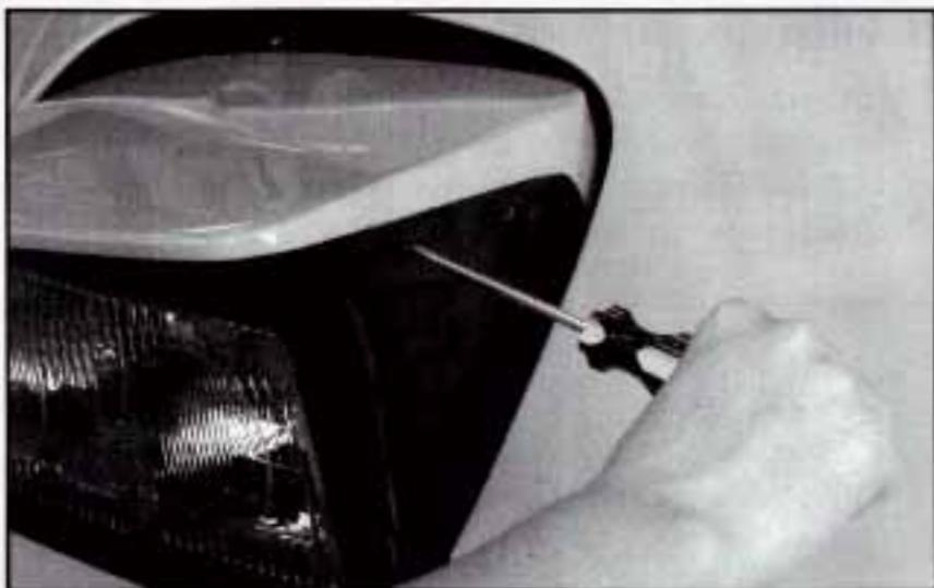
3. Remove the screws on each side of the headlamp bezel.
