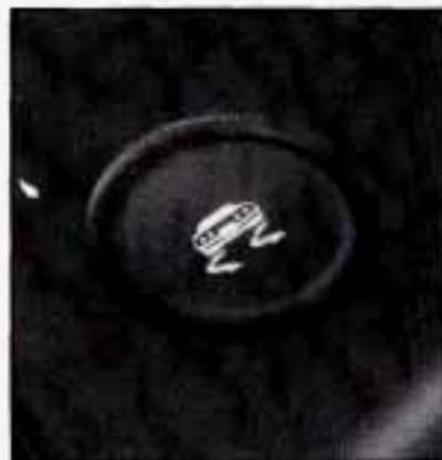
To turn the system off, press the button located on the console. You can turn the system ON or OFF at any time by pressing the TCS switch. The DIC will display the appropriate message when you push the button.
