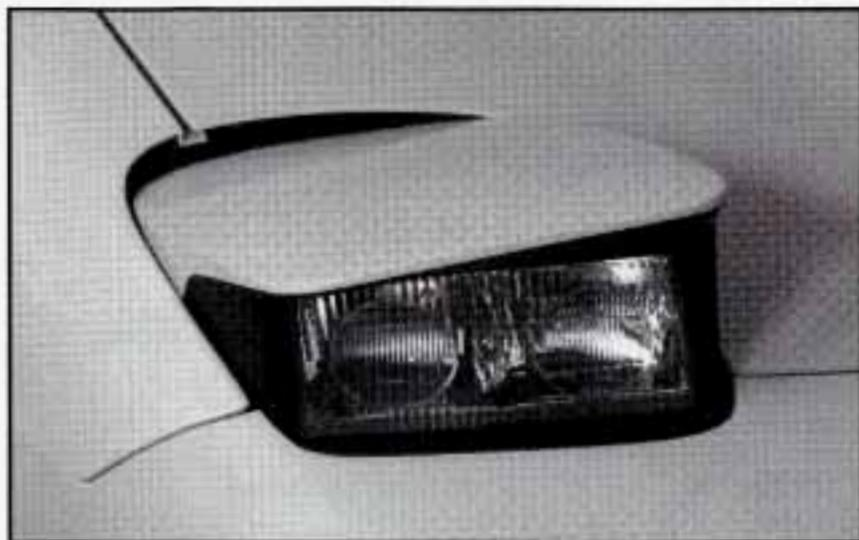
The headlamp doors are designed to open when you turn the headlamps on, and close when you turn the headlamps and parking lamps off. The headlamp doors will stay open if the headlamps are on and then the headlamp switch is turned back to the parking lamps setting.
