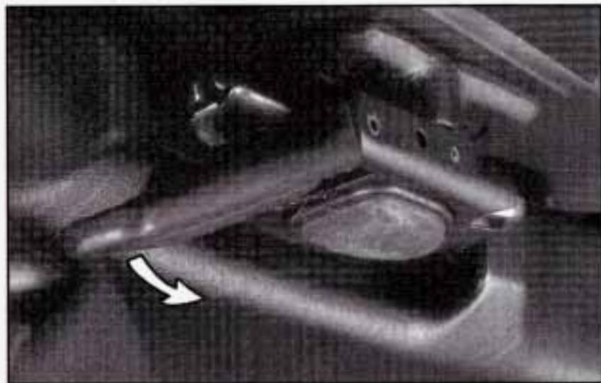
4. To unlock the front of the roof panel, pull down each of the front handles. Grasp the handles with your fingers and pull each toward you. Complete a 180° rotation toward the center of the vehicle. Then push up on each of the handles.
