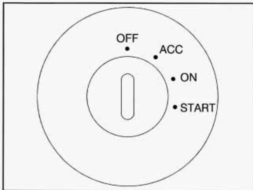
With the key in the ignition switch, you can turn the switch to four positions.
