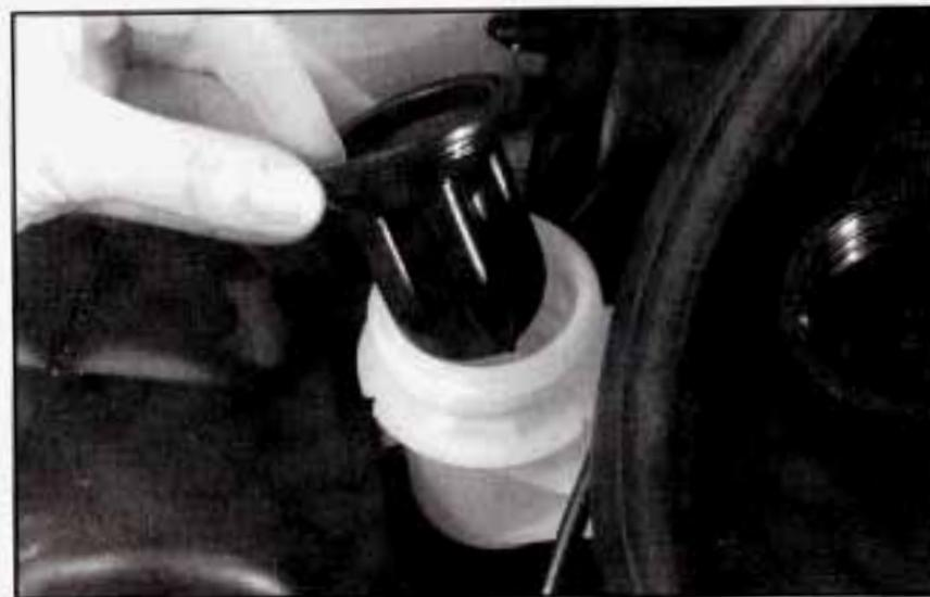
Fluid should be added if the fluid level is below the step on the inside of the reservoir. There are additional instructions on the reservoir cap.
