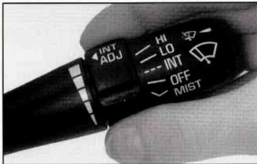
You can control the windshield wipers by moving the lever with the wiper symbol on it. This lever is located on the right side of your steering column.
