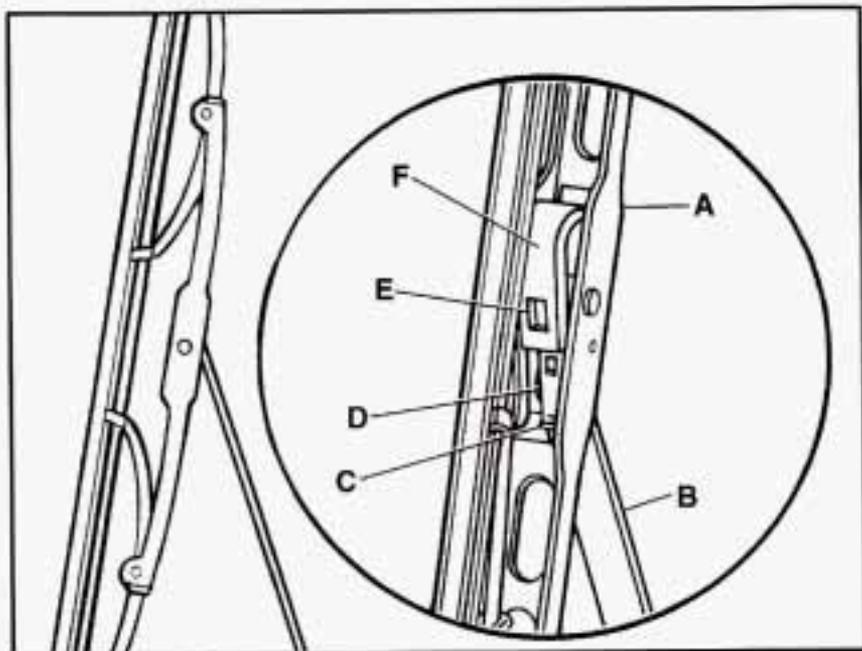
3. Press down on the blade assembly pivot locking tab. Pull down on the blade assembly to release it from the wiper arm hook.
