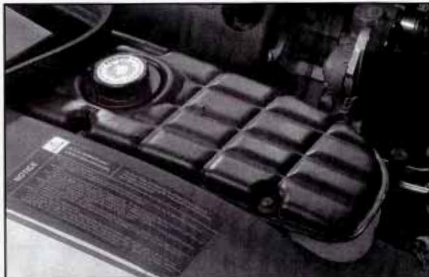
The coolant surge tank is in the engine compartment behind the headlamp on the passenger's side.
