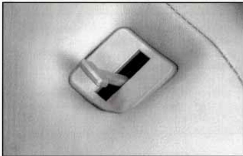
Both seatbacks fold forward to give you access to the rear area. To fold a seatback forward, lift this latch and pull the seatback forward. The seatback will lock down in this position. To unlock, lift up on the latch and push the seatback rearward. When you return the seatback to its original position, make sure the seatback is locked.
