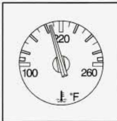
This gage shows the engine coolant temperature. If the gage pointer moves into the shaded area, your engine is too hot!
