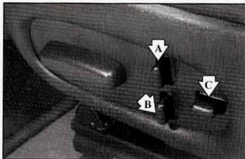
In addition to the power seat control, there are three other switches that help you change the shape of your seat. There are two lumbar supports (A and B) for the middle and lower back. There's also a side bolster switch (C) that adjusts the sides of the seat around you to give you more lateral support.
