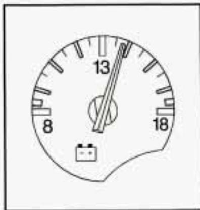
When the key is in the ON position with the engine not running, the voltmeter shows the voltage output of your battery. When the engine is running, it shows the voltage output of the charging system.
