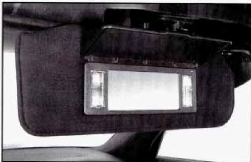
Pull down the sun visor and lift the cover to expose the vanity mirror. When the cover is lifted, the lights will come on automatically, even if the ignition is off.
