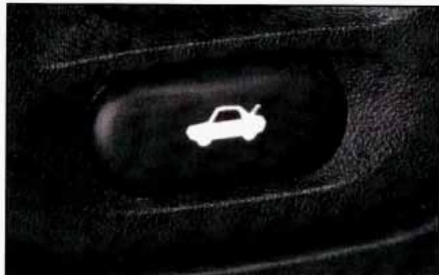
Press the button with the trunk symbol on it, at the left side of the steering column on the instrument panel, to release the hatch from inside your vehicle.
