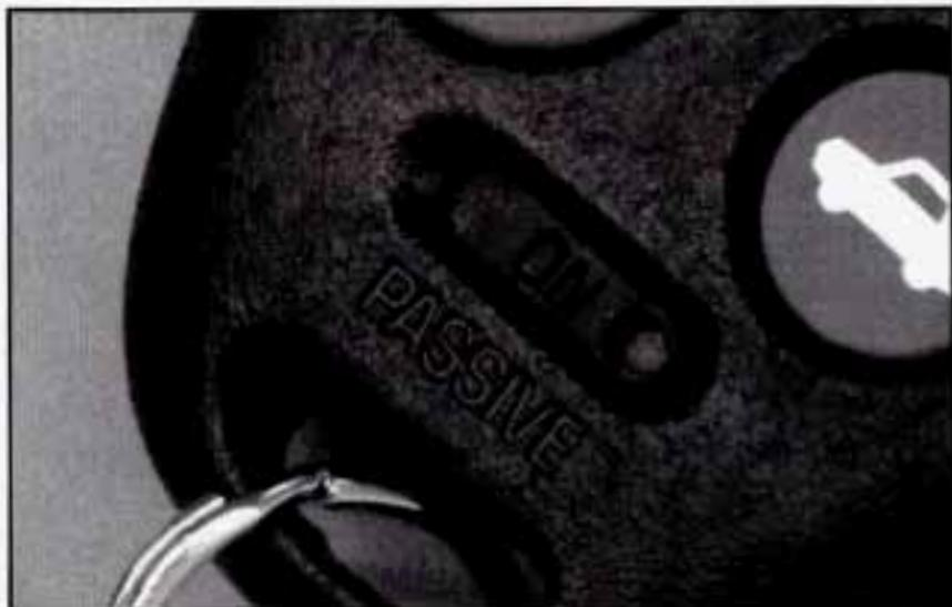
You can turn on the passive feature by moving the transmitter's slider switch to ON. Now, when you move toward your vehicle with the key fob transmitter, the system will automatically disarm your theft-deterrent system and unlock the doors. If it's dark enough outside, your interior lamps will come on.
