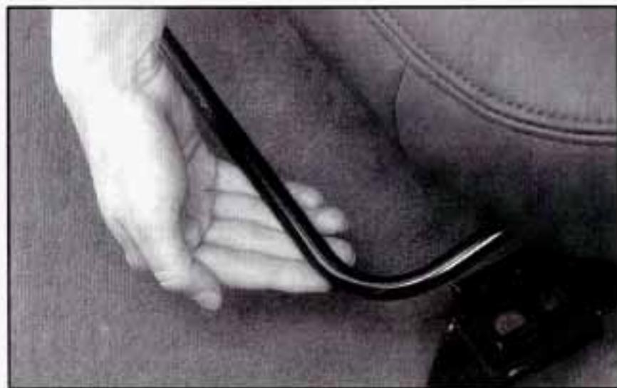
Pull up on the lever in front of the seat to unlock it. Slide the seat to where you want it. Then release the lever and try to move the seat with your body to make sure the seat is locked into place.
