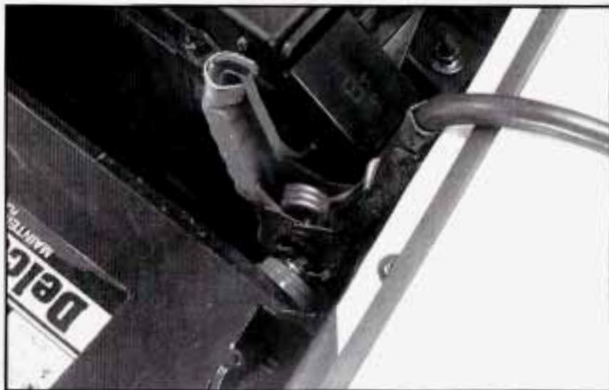
6. Positive (+) goes to positive (+) and negative (-) goes to negative (-) or a metal engine part. Connect the red positive (+) cable to the positive (+) terminal of the vehicle with the dead battery. Use a remote positive (+) terminal if the vehicle has one.
