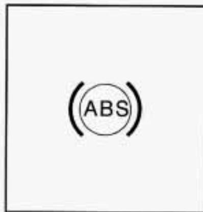
With the anti-lock brake system, the light will come on when you start your engine and may stay on for several seconds. That's normal.
