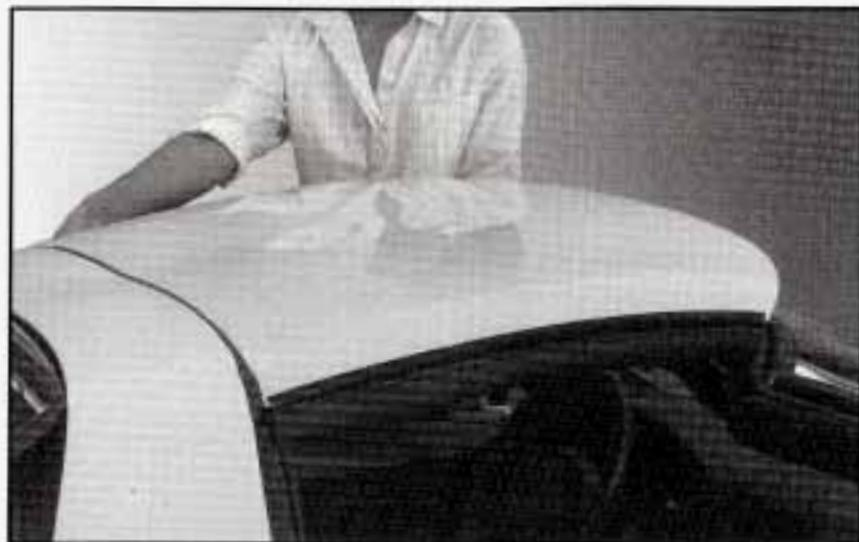
7. Stand on one side of the vehicle and, if necessary, have your helper stand on the other side. Together, carefully lift the front edge of the panel up and forward, and out of the vehicle opening.
