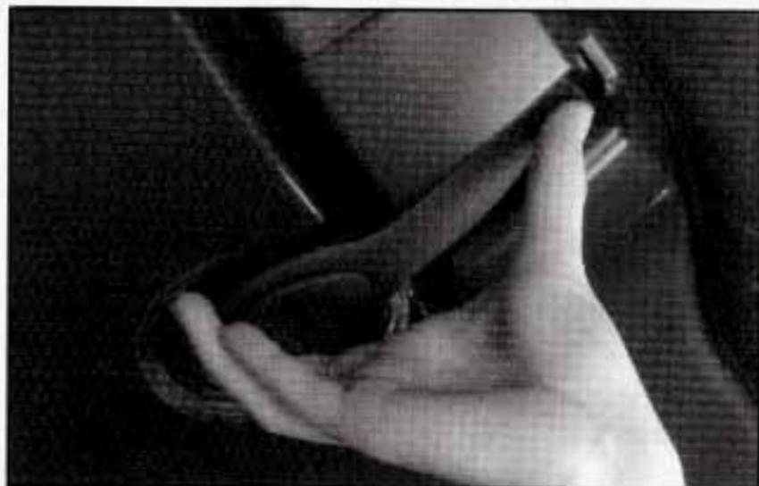
5. To unlock the rear of the roof panel, press the latch release button with your thumb and pull down the latch lever with your fingers.
