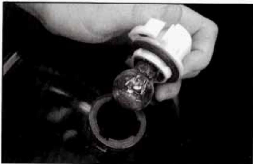
4. Remove the bulb from the socket.
