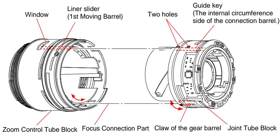
8. After inserting, check that the position is as shown in the figure.
