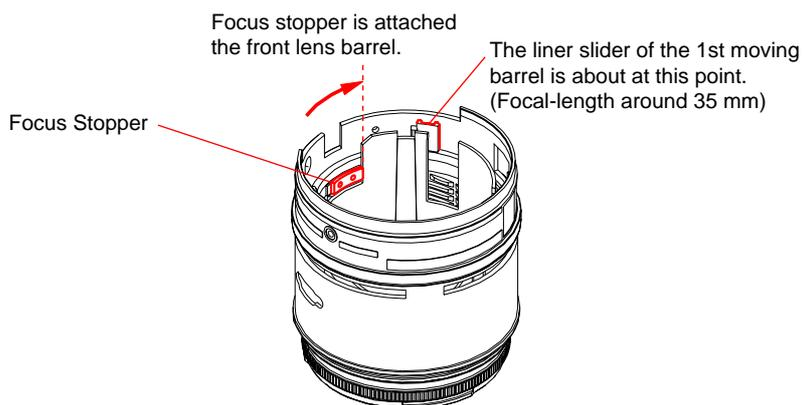
6. Match the positions of the linear slider positioned at the window of the zoom control tube block and the guide key positioned at two holes of joint tube block.
