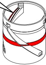
2. Match the positions of joint tube block and zoom cam barrel, and insert the zoom cam barrel into the joint tube block to the end as shown in the figure.
