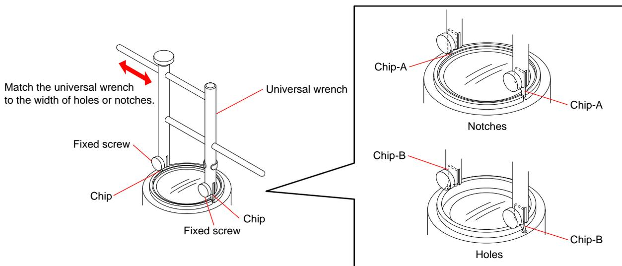
When top of tip does not reach holes or notches because the fixed screw becomes obstructive, replace the fixed screw to below.
