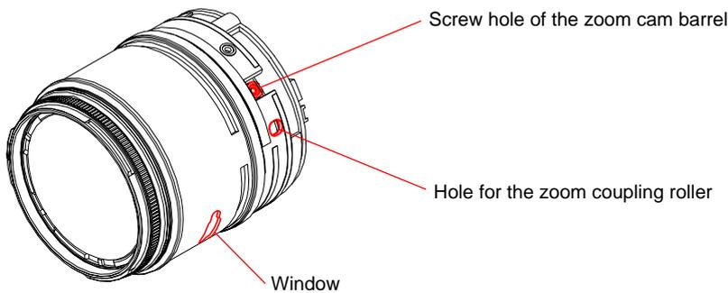
9. Turn the zoom barrel until the screw hole of the zoom cam barrel is seen from the hole of the zoom barrel as shown in the figure.
