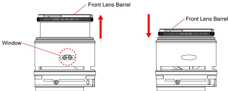
5. Check that the position of the zoom control tube block is as shown in the figure when seeing the inside in the state of step 4.
