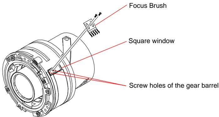
3. Pull the front lens barrel to the telephoto end, and check that the two screw heads are seen from the window.
