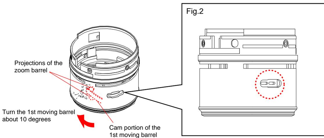
4. Apply the anti-diffusion agent (A-20) to the instruction part of the front lens barrel.
