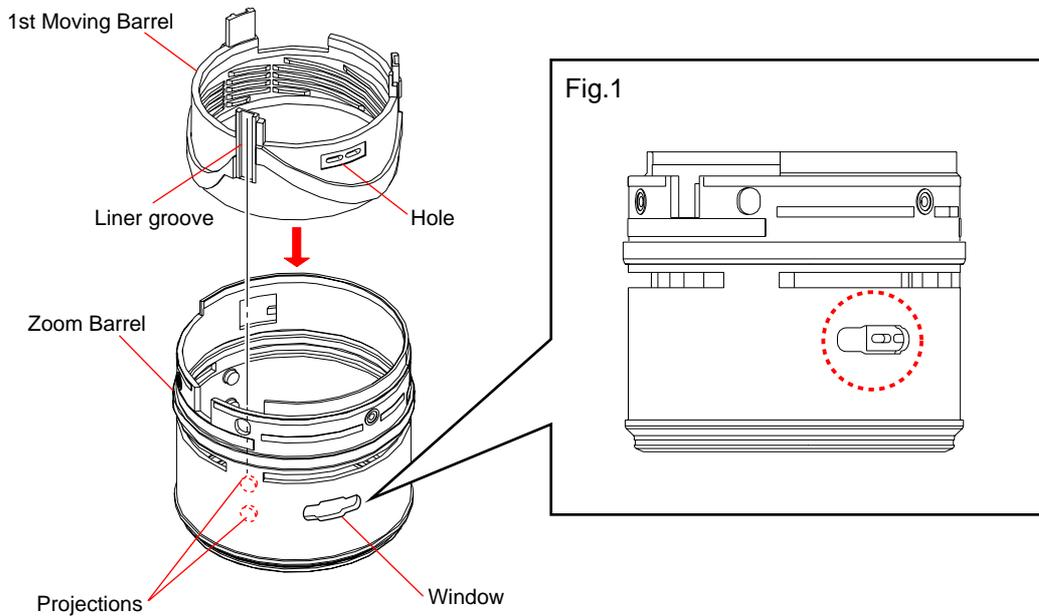
3. Turn the 1st moving barrel to the arrow direction about 10 degrees, and engage the cam part of the 1st moving barrel and projection of the zoom barrel as shown in the figure.
