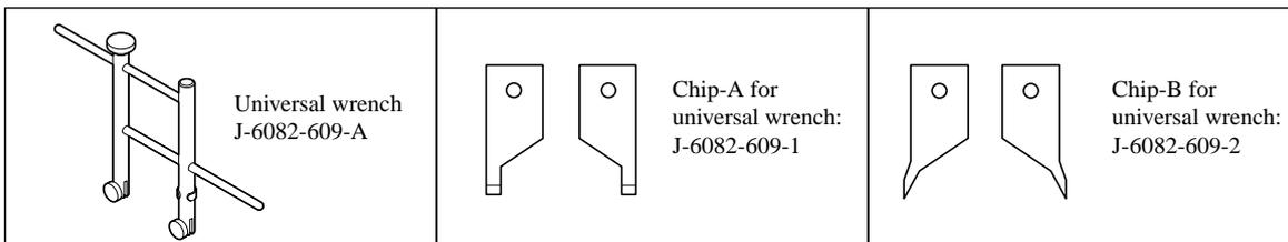
Attach the chip-A or chip-B to the universal wrench.
