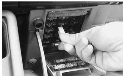
Figure 15-10. The fuse that supplies power to the ECM is usually located in the main fuse block. Pull this fuse to clear stored codes in OBD I systems. Remember that this will not work with most OBD II systems.
