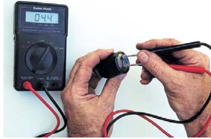
Figure 15-40. Use an ohmmeter to test solenoid and relay windings. Any reading other than the one specified indicates a defective winding.
