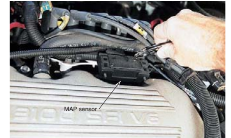
Figure 15-46. When replacing a MAP sensor, disconnect the vacuum line and the electrical connector. Then remove the fasteners and remove the sensor from its mounting.
