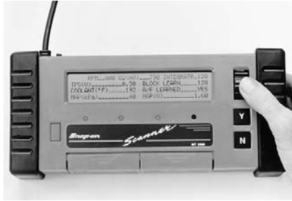
Figure 15-7. This scan tool is widely used. It retrieves trouble codes and displays other engine operating data. This tool also provides information about possible causes of the particular trouble code. (Snap-On)
