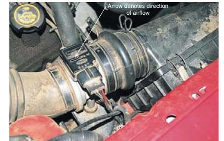
Figure 15-47. When reinstalling an airflow sensor, make sure it is installed in the correct direction. Note the arrow on this sensor, which indicates the direction of airflow
