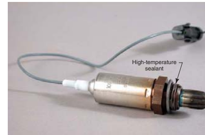
Figure 15-45. If recommended, apply a thin coat of specified sealant to the oxygen sensor threads.
