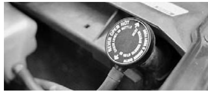
Figure 15-49. Loosen the radiator cap before servicing any part of the cooling system.
