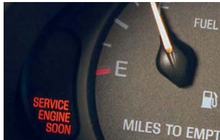
Figure 15-3. The check engine or malfunction indicator light (MIL) is the first place to look when diagnosing any problem. Check the status of this light while test driving the vehicle. (Toyota)
