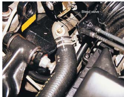
Figure 15-50. After the coolant temperature sensor has been replaced, it may be necessary to bleed air from the cooling system. Some engines are equipped with bleed valves. This one is located on the thermostat housing.
