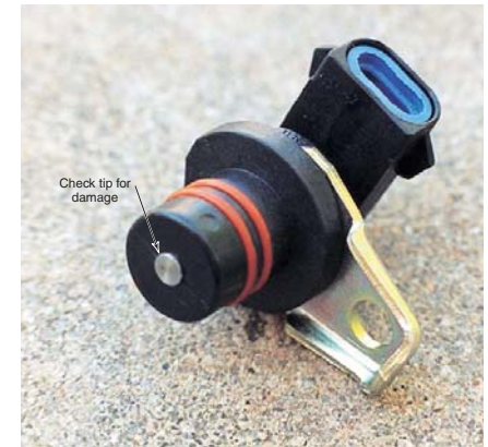
Figure 15-52. After removing a crankshaft or camshaft position sensor, check its tip for signs of damage. If damage is found, be sure to determine and correct the cause before installing a new sensor.
