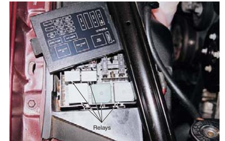
Figure 15-55. Relays are installed in one of several fuse boxes. Be sure that you are replacing the correct relay.
