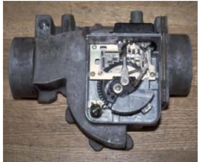
**Figure 25-35** A typical air vane sensor with the cover removed. The movable arm contacts a carbon resistance path as the vane opens. Many air vane sensors also have contacts that close to supply voltage to the electric fuel pump as the air vane starts to open when the engine is being cranked and air is being drawn into the engine.
