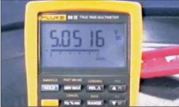
**P19-7** Select DC volts and turn the ignition key on (engine off). The meter reads slightly over 5 volts, confirming the computer is supplying the reference voltage to the TP sensor.
