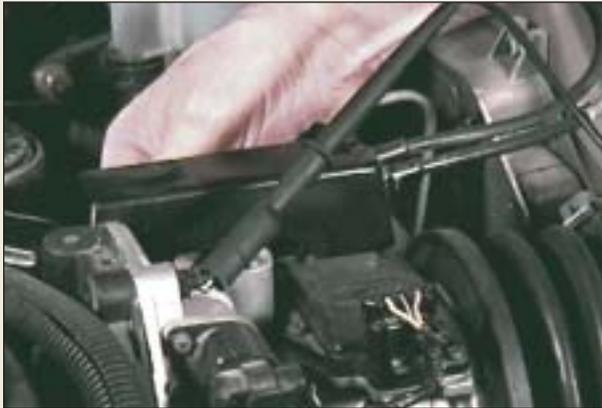
**P19-13** Slowly move the throttle from idle speed to wide open and back to idle speed position. For best results, this test should be performed by depressing the accelerator pedal. This puts the same forces on the sensor as occurs during normal driving.
