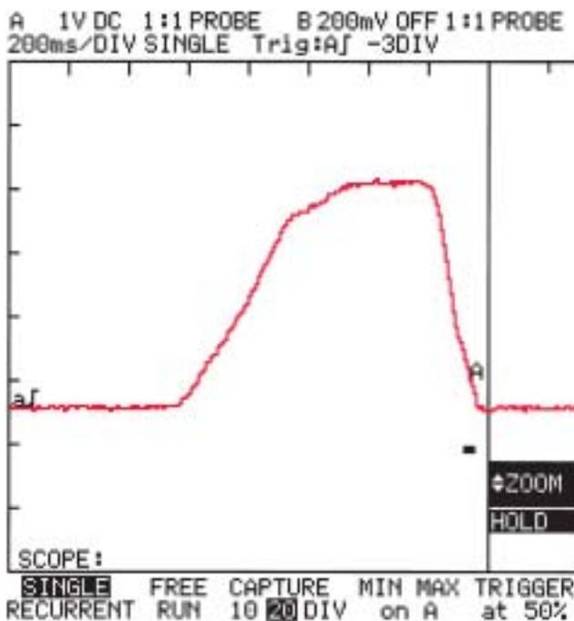
**Figure 25–28** A typical waveform of a TP sensor signal as recorded on a DSO when the accelerator pedal was depressed with the ignition switch on (engine off). Clean transitions and the lack of any glitches in this waveform indicate a good sensor. (Courtesy of Fluke Corporation)
