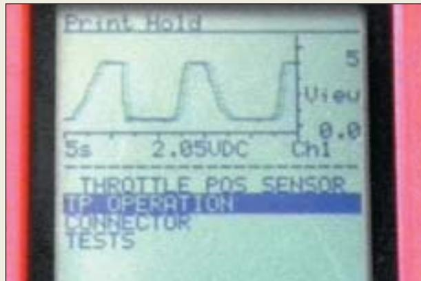
**P19-18** After attaching the meter leads to the signal wire and ground (ignition key on, engine off), the graphing multimeter shows the waveform of the voltage signal as the throttle is depressed, released, and depressed again. These are normal for a TP sensor. A fault would show as a vertical line or dip in the waveform.
