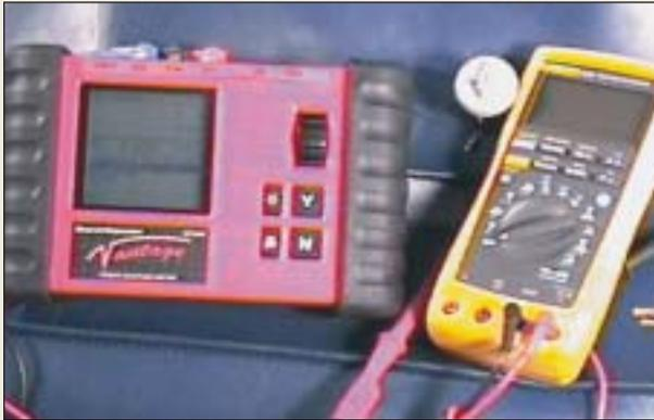
**P19-1** Besides a scan tool, other equipment that can be used to check a throttle position (TP) sensor includes a scope or graphing multimeter, a digital multimeter equipped with MIN/MAX function, and T-pins to safely backprobe the sensor wires.
