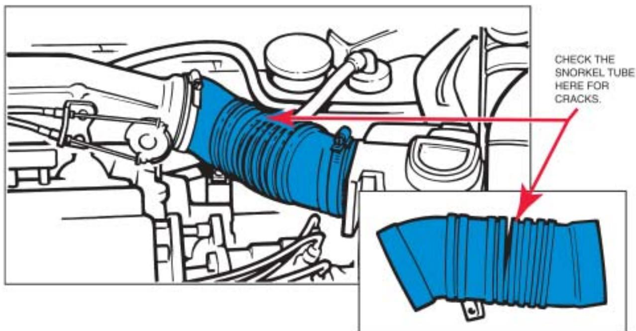
**Figure 25-38** Carefully check the hose between the MAF sensor and the throttle plate for cracks or splits that could create extra (false) air in the engine that is not measured by the MAF sensor.
