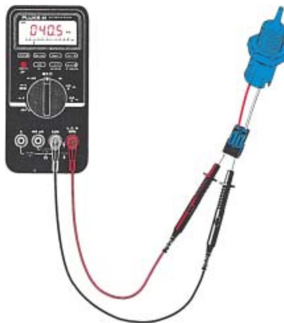
**Figure 25–22** Measuring the resistance of the ECT sensor. The resistance measurement can then be compared with specifications. (Courtesy of Fluke Corporation)
