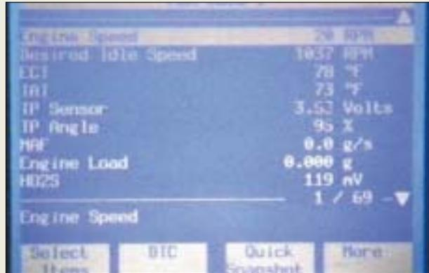
**P19-4** A scan tool can be used to observe the output voltage and the calculated percentage (%) of throttle opening.
