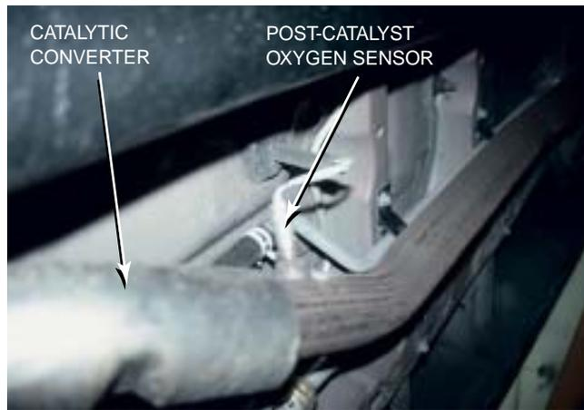
**Figure 25–32** Most 1996 and newer vehicles use an oxygen sensor behind the catalytic converter. The purpose of the oxygen sensor is to sense the percentage of oxygen in the exhaust to check the efficiency of the catalytic converter.
