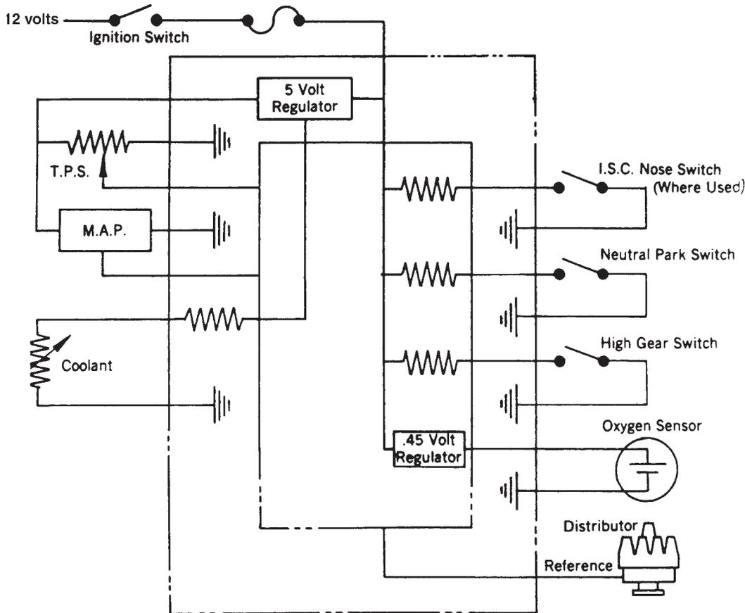
Figure 25-9 Basic computer inputs. (Courtesy General Motors)
