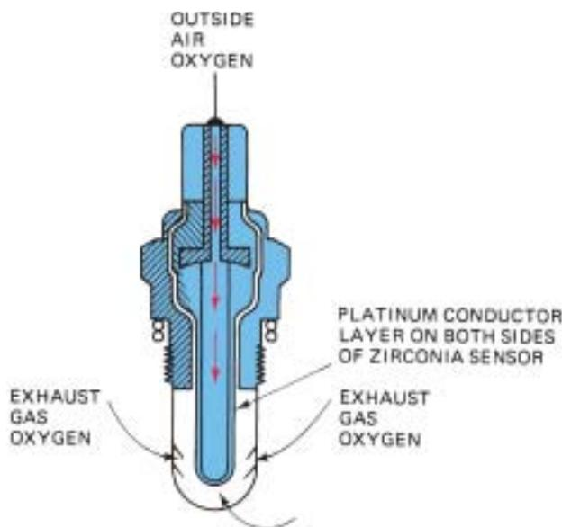
**Figure 25-19** A cross-sectional view of a typical zirconia oxygen sensor.
