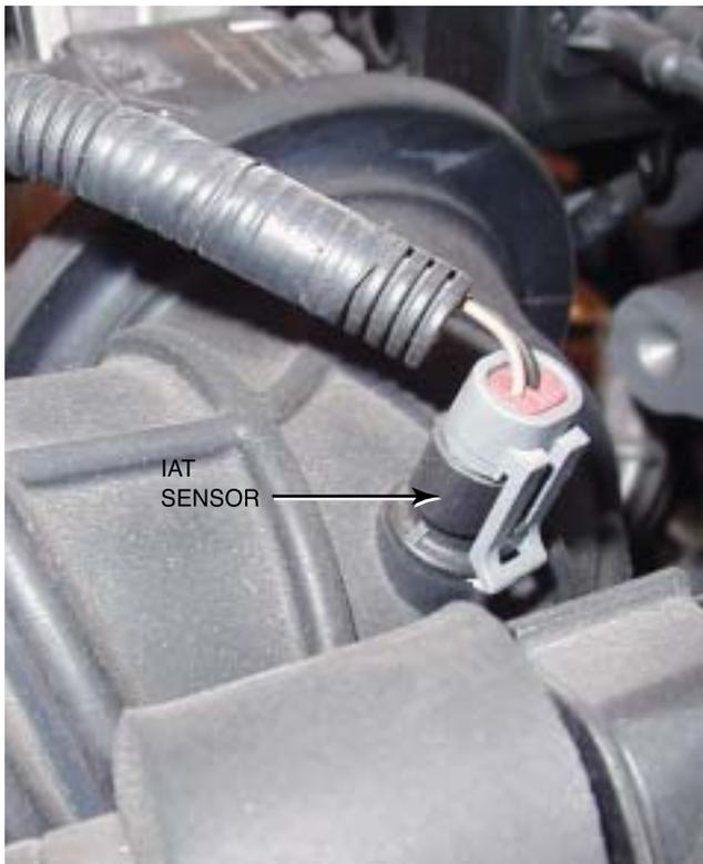
**Figure 25–25** The IAT sensor on this General Motors 3800 V-6 engine is in the air passage duct between the air cleaner housing and the throttle plate.
