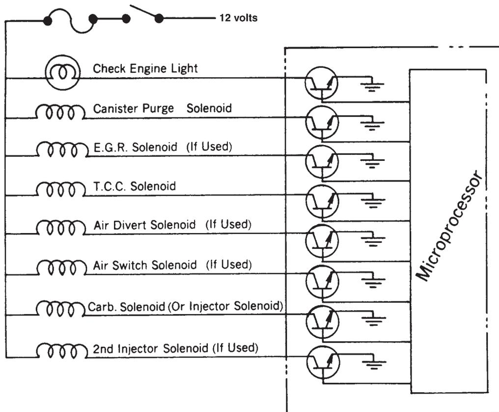
Figure 25-21 Basic computer outputs. (Courtesy General Motors)
