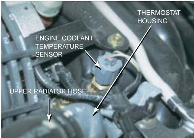
**Figure 25–14** A typical engine coolant temperature (ECT) sensor. ECT sensors are located near the thermostat housing on most engines.
