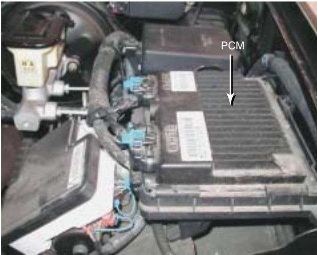
**Figure 25-7** This powertrain control module (PCM) is located under the hood on this pickup truck.
