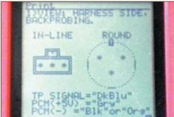
**P19-17** The Vantage has a built-in database that can be accessed to show connector position and wire colour information.
