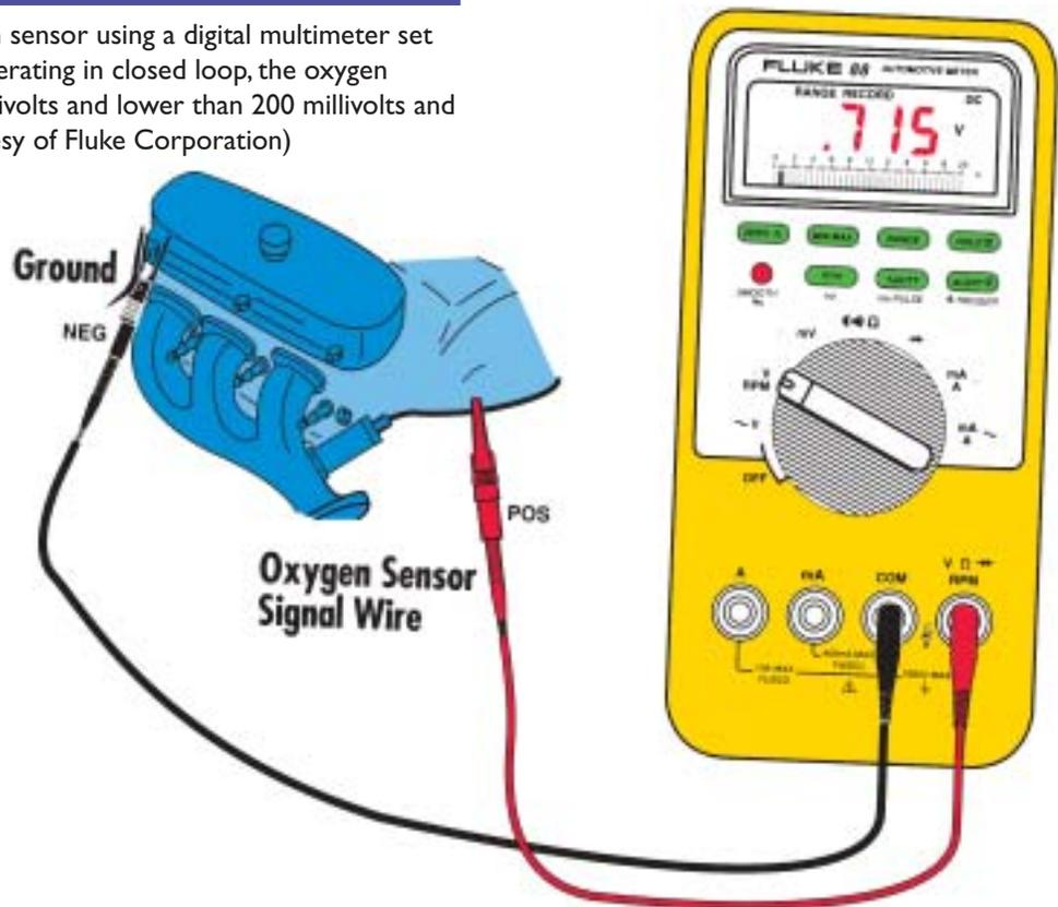
the engine running. A good oxygen sensor should be able to produce a value of less than 300 millivolts and a maximum voltage above 800 millivolts. Replace any oxygen sensor that fails to go above 700 millivolts or lower than 300 millivolts.
