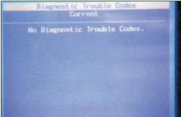
**P19-3** A scan tool display showing no diagnostic trouble codes (DTCs). A fault could still exist even though a diagnostic trouble code is not set—it depends on what type of fault and when it occurs.
