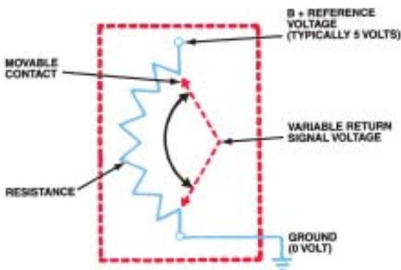
**Figure 25-2** A potentiometer uses a movable contact to vary resistance and send an analog signal.
