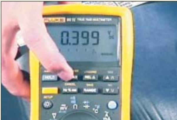
**P19-15** Pushing the MIN/MAX button shows the minimum voltage the meter recorded during the test (0.399 volts).
