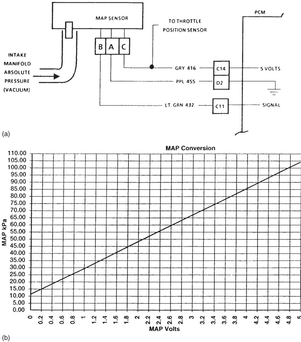
**Figure 25-13** (a) Schematic of a typical manifold absolute pressure (MAP) sensor circuit. (b) As manifold pressure (vacuum) changes, the voltage signal to the computer also changes. (Courtesy General Motors)
