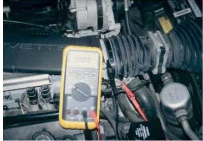
**Figure 25–30** Checking the voltage drop between the TP sensor ground and a good engine ground with the ignition on (engine off). A reading of greater than 0.6 V (600 mV) represents a bad computer ground.
