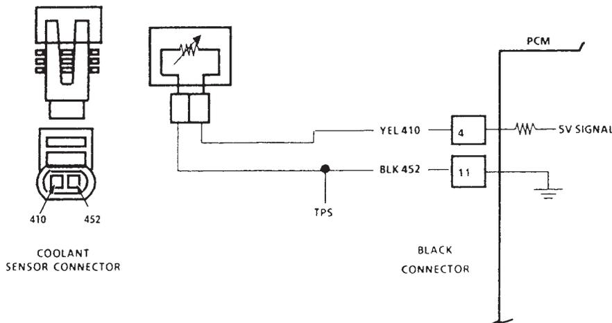
**Figure 25–16** Schematic of a typical engine coolant temperature sensor circuit. The computer measures the voltage signal between the PCM resistor and the ECT resistance. (Courtesy General Motors)
