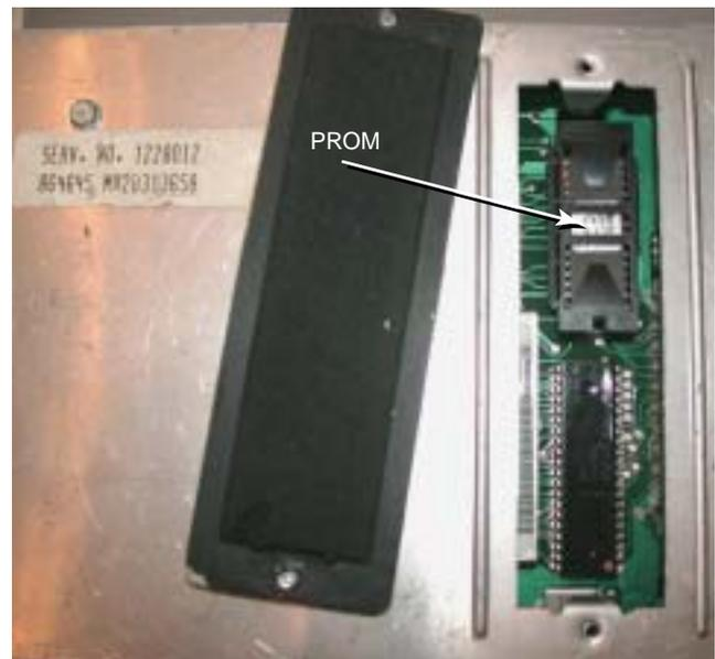
**Figure 25-5** A replaceable PROM used in a General Motors computer. Notice that the sealed access panel has been removed to gain access.
