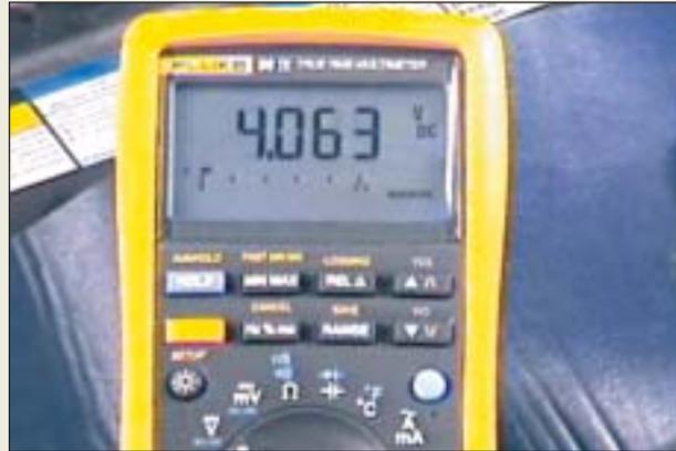
**P19-14** The high reading for this sensor was 4.063 volts.
