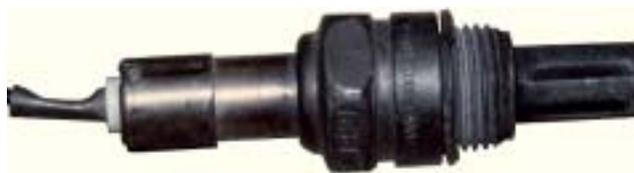
**Figure 25-18** Typical zirconia oxygen sensor.
