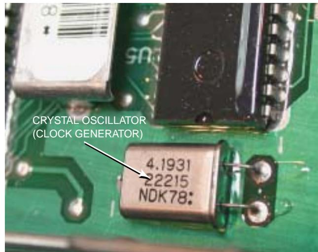
**Figure 25–6** The clock generator produces a series of pulses that are used by the microprocessor and other components to stay in step with each other at a steady rate.
