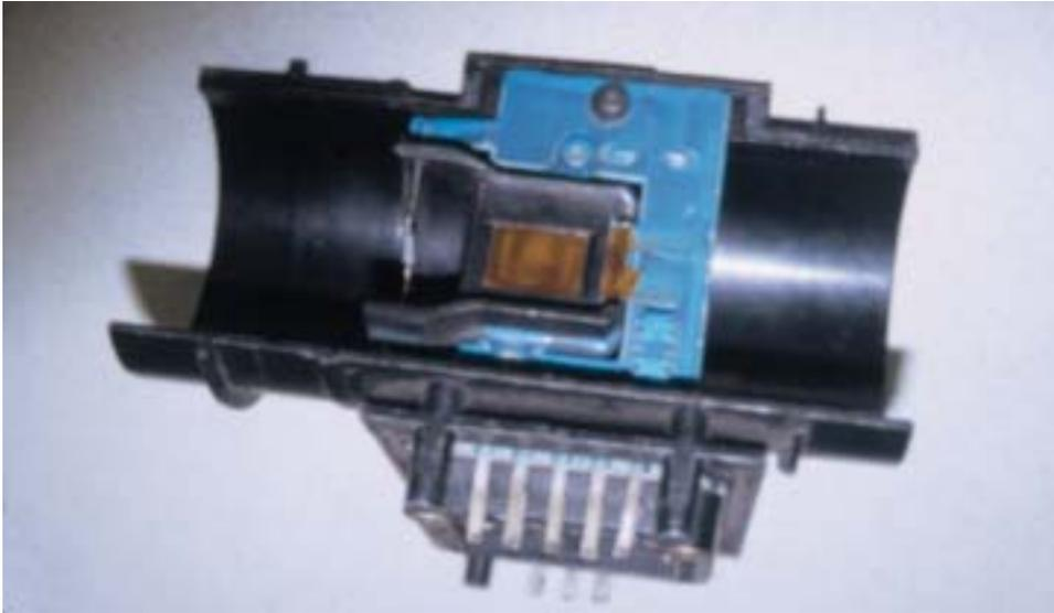
**Figure 25-36** A GM hot film mass air flow (MAF) sensor that has been taken apart. The electronic circuit measures the cooling effect of the air entering the engine and generates a frequency output signal that is proportional to the amount of air passing through the sensor.
