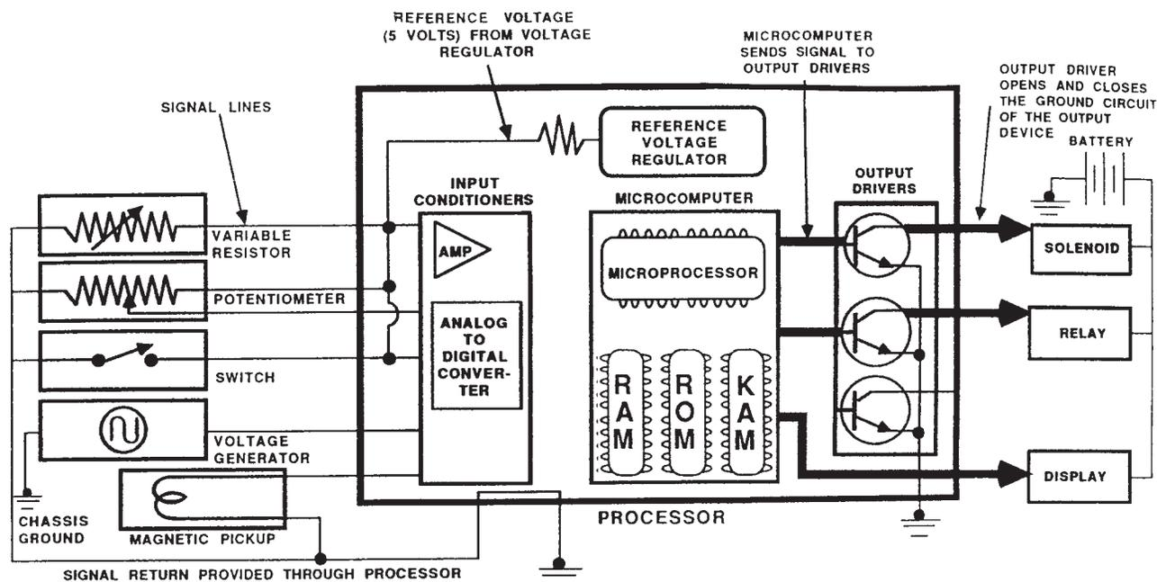
**Figure 25-20** Microprocessor schematic showing input, processing, and output. Note that input sensors operate from a 5 volt reference signal and the output devices operate from battery voltage. (Courtesy Ford Motor Co.)
