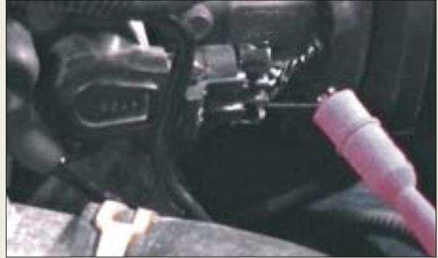
**P19-8** Another important step when testing a TP sensor is to verify that the ground circuit is okay. To check the ground of the TP sensor, carefully backprobe the ground wire at the TP sensor connector (black on this General Motors vehicle) and connect the red meter lead to the T-pin.
