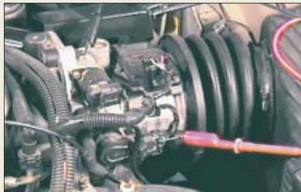
**P19-6** Connect the red lead from the digital multimeter to the T-pin and attach the black meter lead to a good, clean engine ground.
