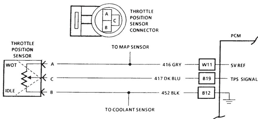
**Figure 25-11** Schematic of a typical throttle position (TP) sensor circuit. Movement of the wiper on the potentiometer sends a voltage signal (0.5 to 4.5 volts) to the computer. (Courtesy General Motors)
