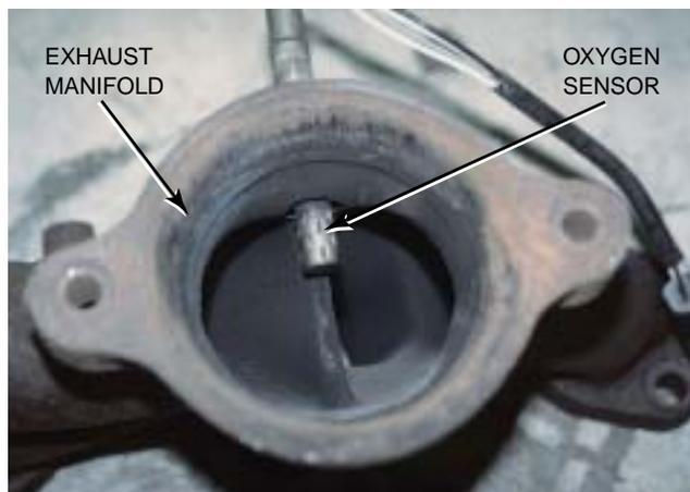
**Figure 25-17** Many fuel control oxygen sensors are located in the exhaust manifold near its outlet so that the sensor can detect the presence or absence of oxygen in the exhaust stream for all cylinders that feed into the manifold.
