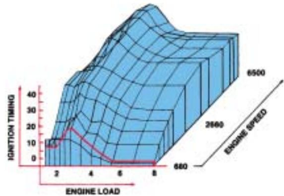
**Figure 25-4** Typical ignition timing map developed from testing and used by the vehicle computer to provide the optimum ignition timing for all engine speeds and load combinations.
