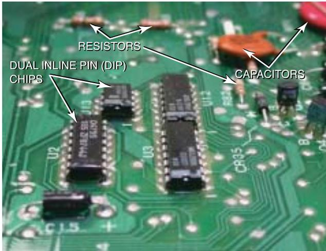
**Figure 25-3** Many electronic components are used to construct a typical vehicle computer. Notice all of the chips, resistors, and capacitors that are used in this computer.
