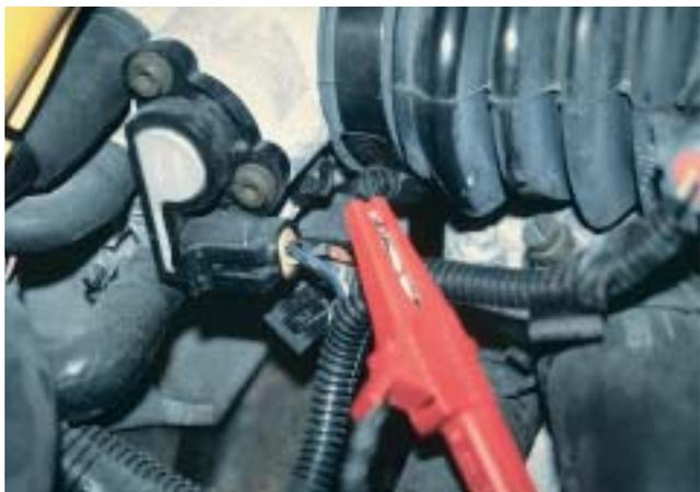
**Figure 25–27** A meter lead connected to a T-pin that was gently pushed along the signal wire of the TP sensor until the point of the pin touched the metal terminal inside the plastic connector.
