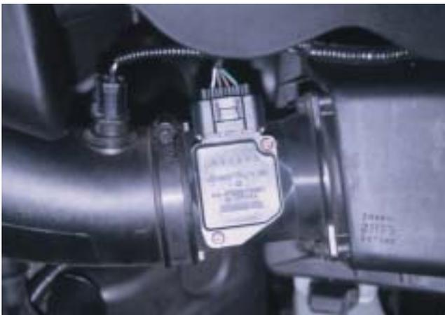
**Figure 25-37** A typical hot wire MAF sensor located between the air filter and the throttle plate.
