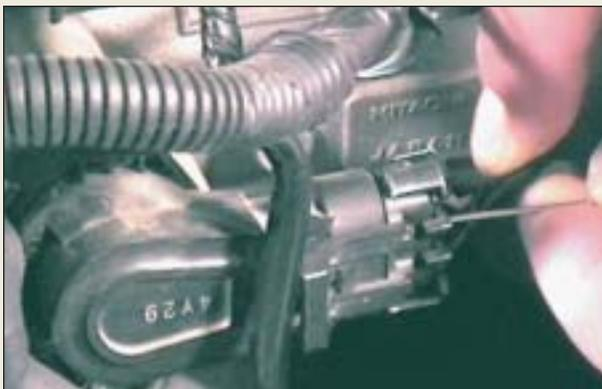
**P19-5** Most throttle position sensors use a 5 volt reference voltage from the computer. To test that this signal is available at the sensor, carefully backprobe the 5 volt reference (grey on this General Motors vehicle) wire at the connector on the TP sensor. Simply push the T-pin alongside the wire until it touches the metal terminal inside the connector.
