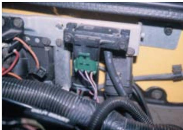
**Figure 25-12** This MAP sensor is installed on the bulkhead with a vacuum hose attached that runs to the intake manifold. Some MAP sensors are attached directly to the intake manifold.
