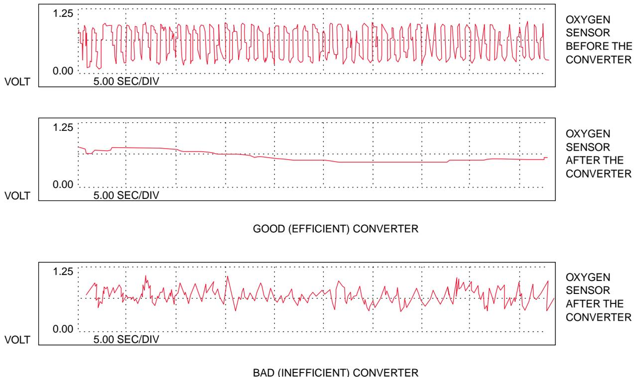
**Figure 25–33** The post–catalytic converter oxygen sensor should display very little activity if the catalytic converter is efficient.
