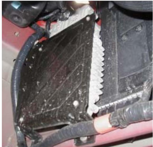
**Figure 25-8** This PCM on a Chrysler vehicle can only be seen by hoisting the vehicle because it is located next to the radiator in the airflow to help keep it cool.
