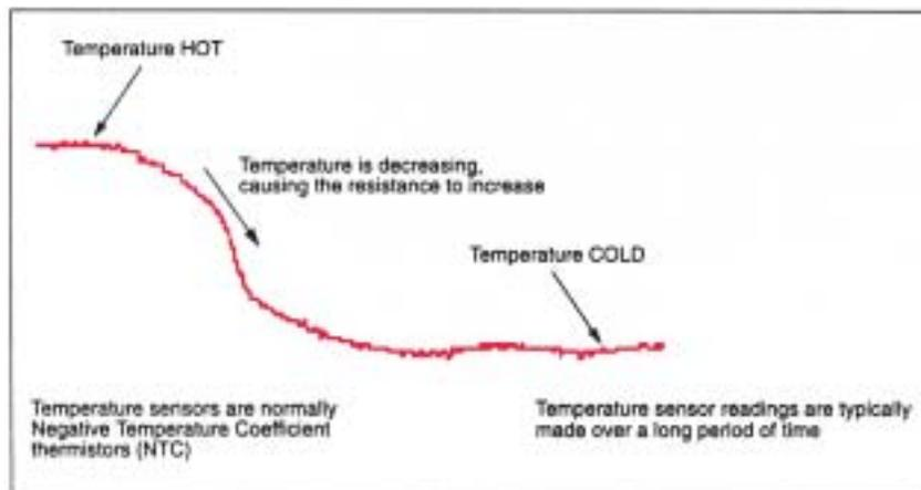
If resistance values match the approximate coolant temperature and there is still a coolant sensor trouble code, the problem is generally in the wiring between the sensor and the computer. Always consult the manufacturer's recommended procedures for checking this wiring. If the resistance values do not match, the sensor may need to be replaced.
