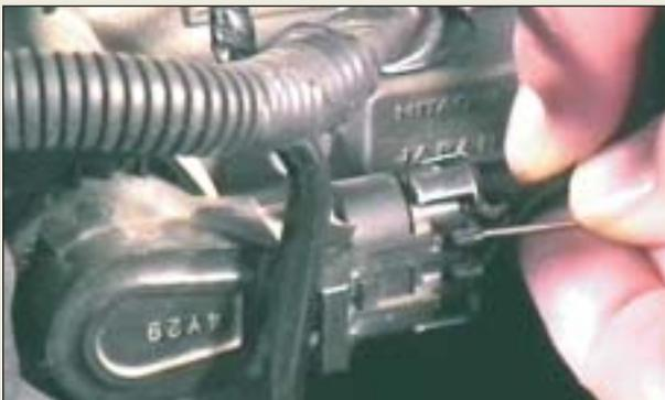
**P19-11** To measure the signal voltage, backprobe the signal wire (dark blue on this General Motors vehicle).
