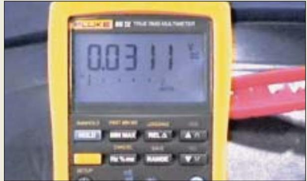
**P19-10** With the ignition on (engine off) and the digital meter still set to read DC volts, read the voltage drop of the TP sensor ground. The voltage drop is the difference in voltage between the leads of the meter. General Motors specifies that this voltage drop should not exceed 35 mV (0.035 V). This TP sensor ground shows 31.1 mV (0.0311 V).
