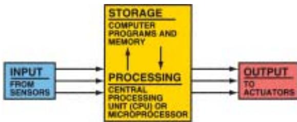
**Figure 25-1** All computer systems perform four basic functions: input, processing, storage, and output.
