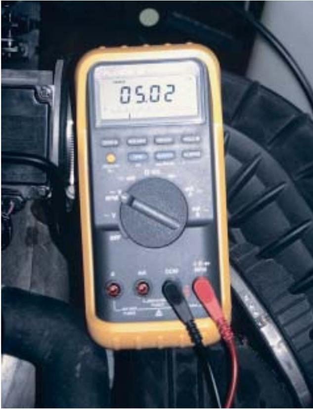
**Figure 25–29** Checking the 5 volt reference from the computer being applied to the TP sensor with the ignition switch on (engine off).
