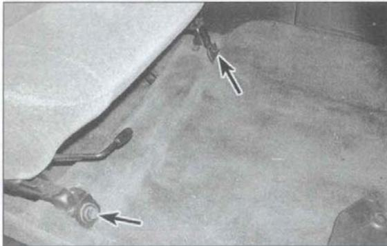
28.1a Remove the two front bolts (arrows) for the front seat . . .
