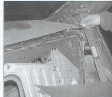
29.3 Pry up the package shelf with a trim tool - slide the tool along between the shelf and the body until you locate the plastic pins, then pry up
