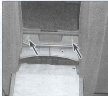
28.3b Fold down the center armrest in the back seat and remove these bolts (arrows) . . .
