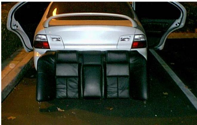
To remove the rear seats, start with the horizontal cushion. Simply pull the retainer ring forward while pulling up on the seat. There are two retainer rings, one on the left and one on the right. See picture 28.3a from page 11-18 of the Haynes manual below (a full scan of page 11-18 of the Haynes manual can be seen at the end of this write-up). Once the two retainer rings are unclipped, pull the front of the lower cushion forward and up, and then remove it from the car.
