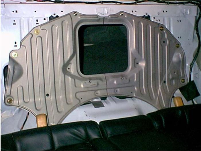
Refer to FSM page BT-15 found at the end of this write-up for removal of the plate. There are eight 10mm bolts spaced equally around the metal plate and two 10mm nuts at the top of the plate.
