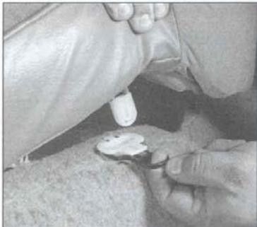
28.3a Pull out on the clip retainer ring while pulling sharply upward to detach the back seat lower cushion
