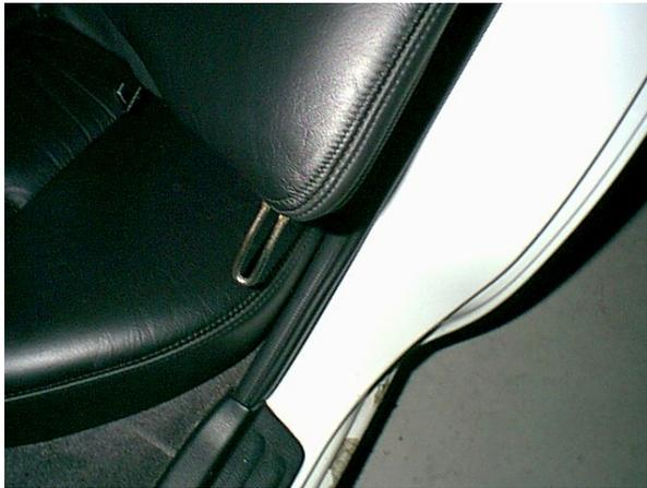
To gain access to the two bolts in the armrest, unhook and pull forward the vinyl gray cloth hanging between the armrest and the pass-through opening. To unhook it, pull straight up on the plastic part attached to the vinyl cloth. It is hooked onto the lower opening of the armrest pass-through. See picture below.
