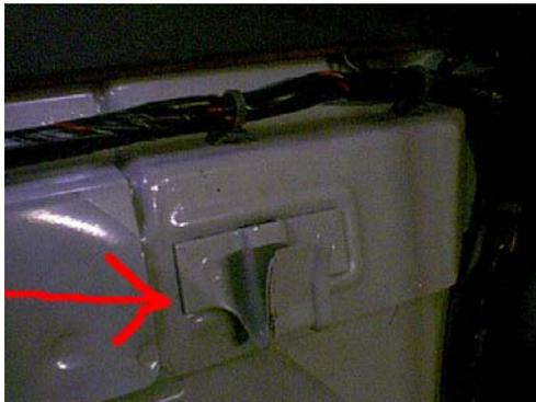
2.) The next step is to remove the metal 'plate' attached to the back wall. You can see the metal plate in picture 29.3, page 11-18, of the Haynes manual (full page 11-18 shown at the end of this write-up) but here is a better picture.
