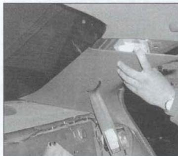
29.2 Pry out the rear roof pillar trim panels, and slide them along the seat belts and out of the way
