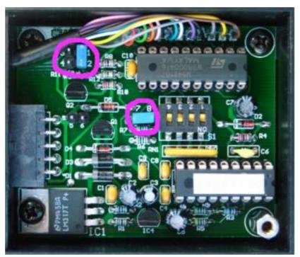
The above photograph shows the jumpers (circled in pink) set to TRE enabled. To disable the TRE, move the jumper 1-2 to 3-4 and remove jumper 7-8.
