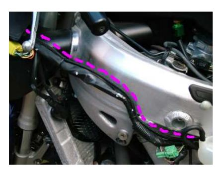
Step 5. The Geartronics control box should be fitted behind the fuse box located under, and in front of, the left handlebar. The control box should be mounted with the connector at the bottom so as to reduce the possibility of water ingress.
