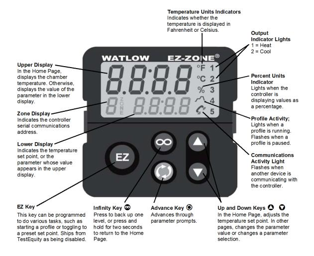
**Temperature Controller Keys and Displays**
