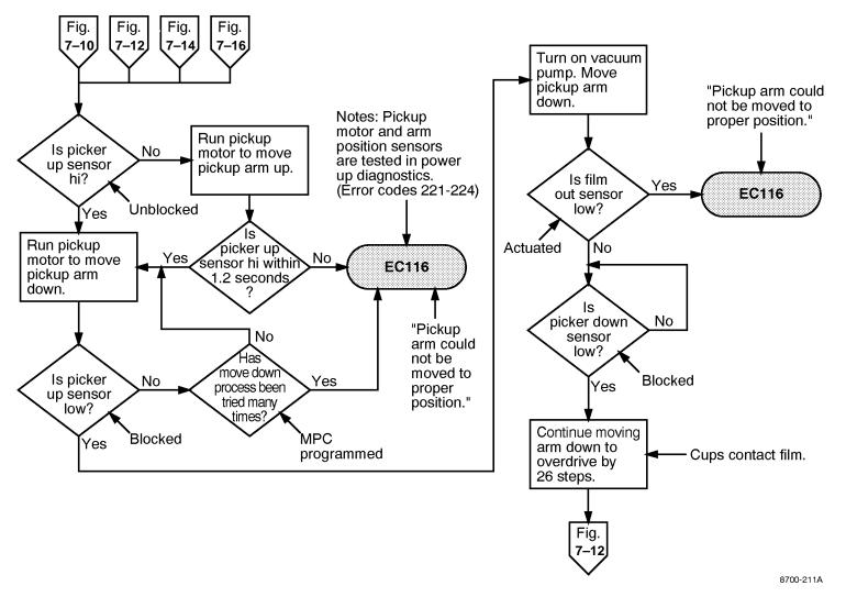
Figure 7-11. Position Pickup Arm Sequence
