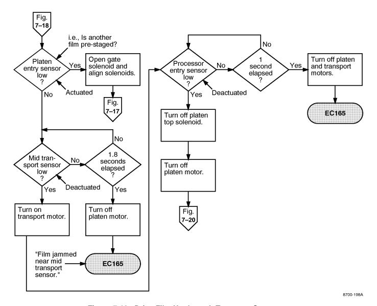
Figure 7-19. Drive Film Up through Transport Sequence
