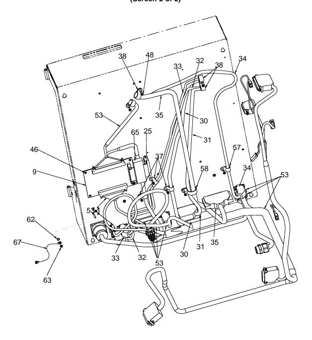
Figure 8-23. Electronics Enclosure Assembly, Dual (Screen 2 of 2)
