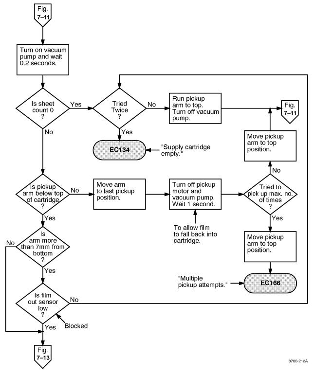
Figure 7-12. Pick Up Film Sequence
