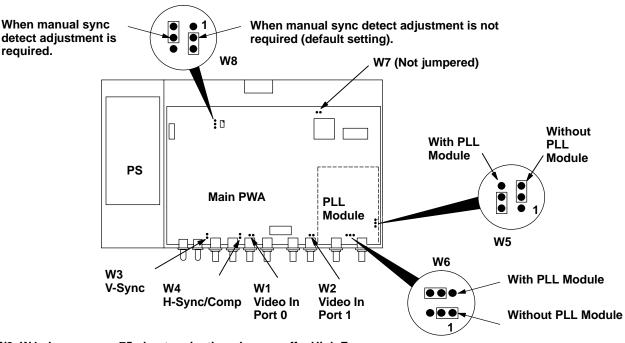
W1, W2, W3, W4: Jumper on = 75 ohm termination; Jumper off = High Z.
