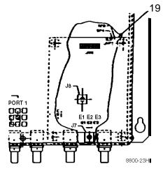
**VEIB** with PLL Module Installed
