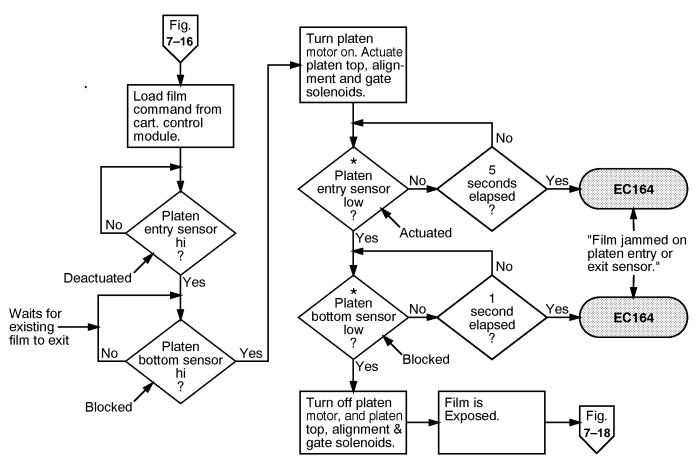
\*While film is in the sensor, the sensor's state is changed.
