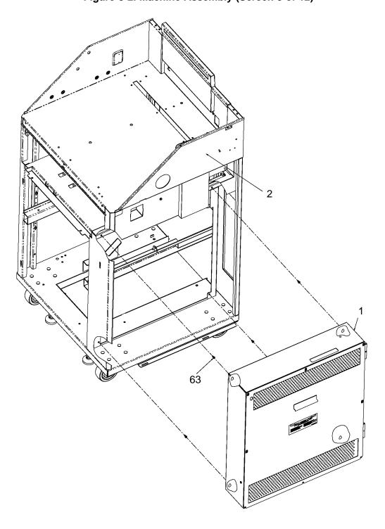
Figure 8-2. Machine Assembly (Screen 3 of 12)
