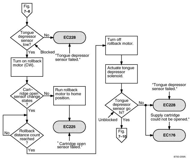
Figure 7-9. Open Cartridge Lid Sequence
