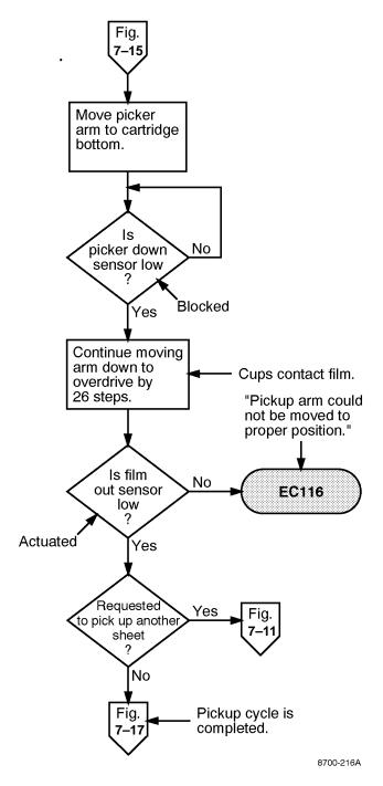
Figure 7-16. Close Out Pickup Cycle Sequence
