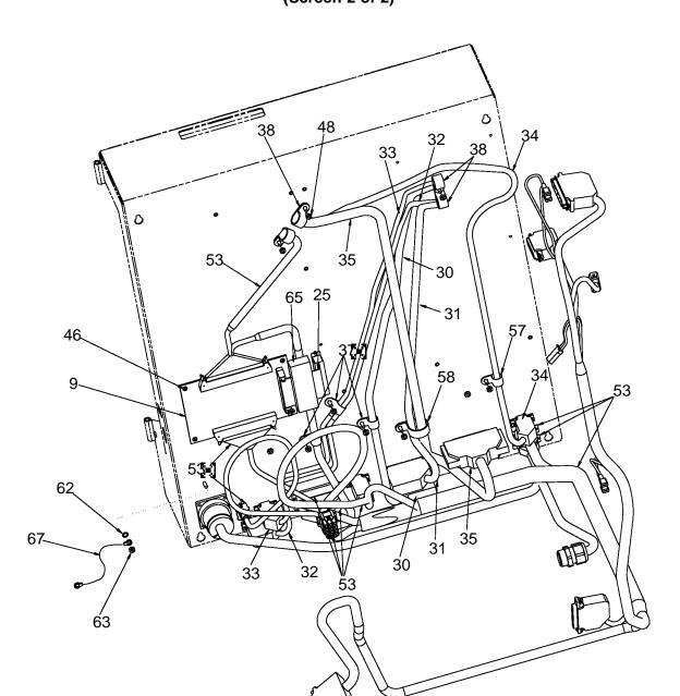
Figure 8-22. Electronics Enclosure Assembly, Standalone (Screen 2 of 2)
