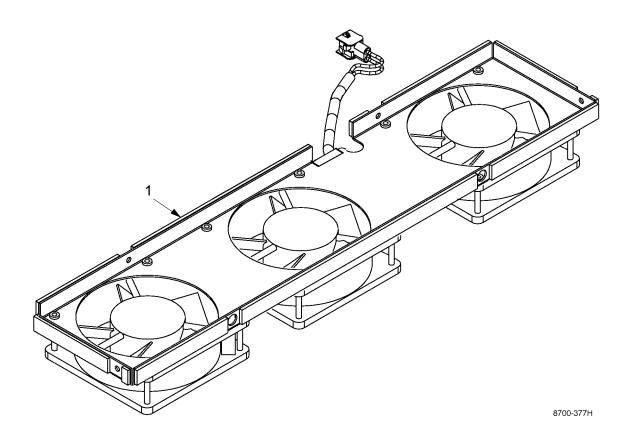
Figure 8-24. Electronics Fan Assembly
