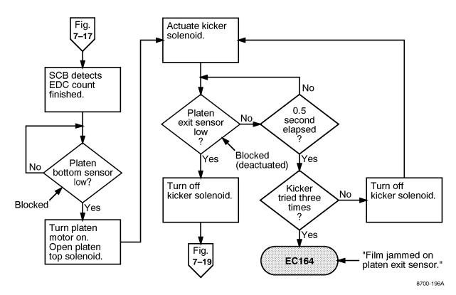
Figure 7-18. Unload Exposed Film from Platen Sequence
