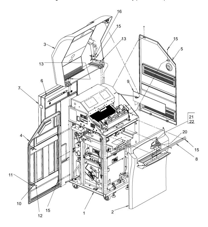
Figure 8-1. Machine and Skins Assembly (Screen 1 of 2)
