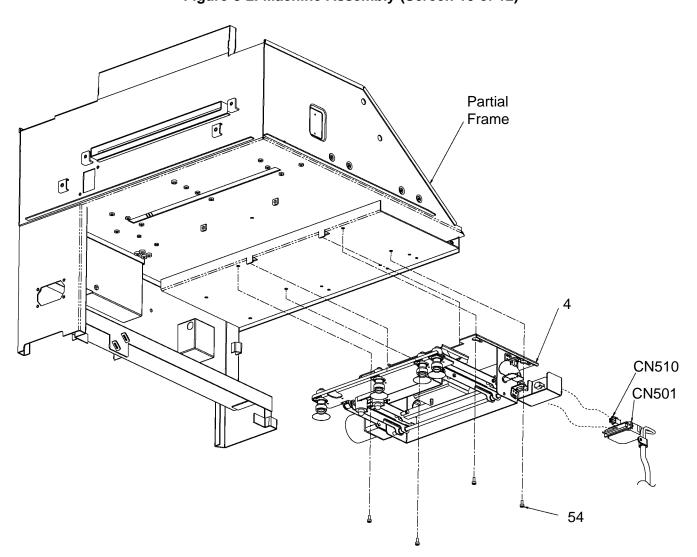
Figure 8-2. Machine Assembly (Screen 10 of 12)
