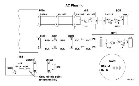
Figure 7-21. Checking 60 Hz Phasing
