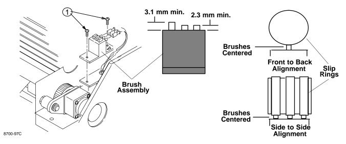
Figure 3-17. Brush to Slip Ring Alignment
