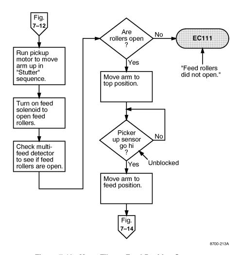
Figure 7-13. Move Film to Feed Position Sequence
