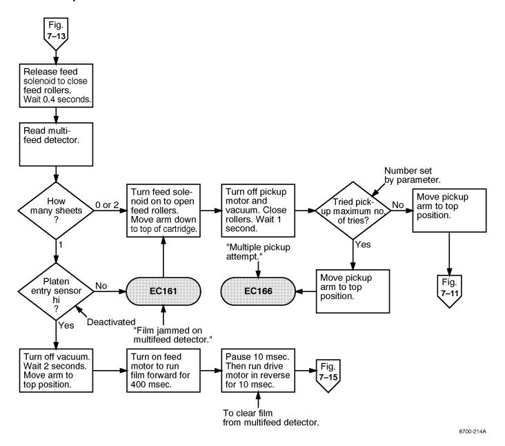
Figure 7-14. Prepare to Feed Film Sequence
