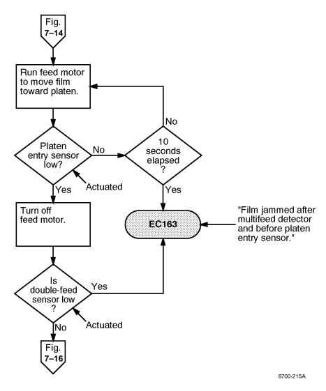
Figure 7-15. Feed Film to Platen Entrance Sequence
