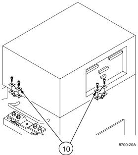
To separate platen and optics module, remove 3 brackets (M3 Allen)
