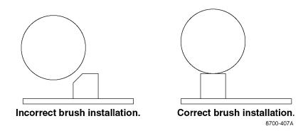
Figure 7-22. Slip Rring/Brush Alignment
