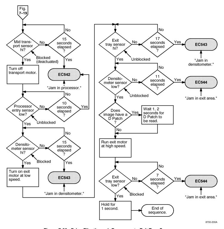
Figure 7-20. Drive Film through Processor to Exit Tray Sequence
