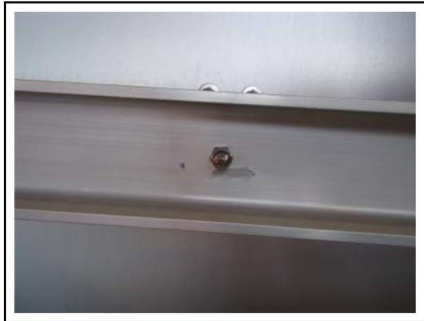
2. Remove the two socket head Allen screws securing the cable plate to the top slider tube.
