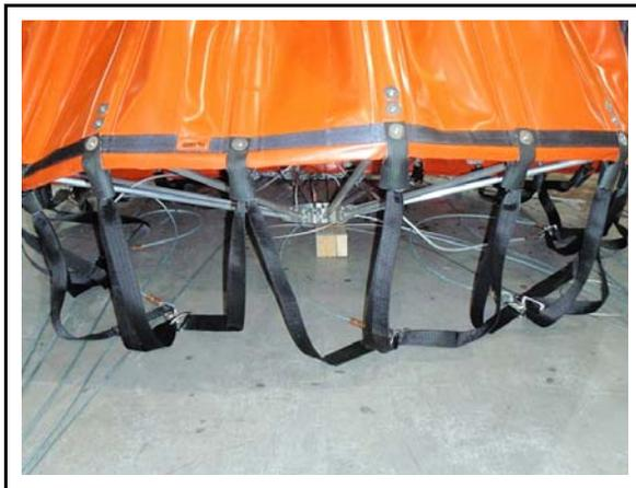
3. Go to the bottom of the bucket and lift. If the bucket is a Torrentula or Torrentula Powerfill, two people may be required to lift the bucket.
