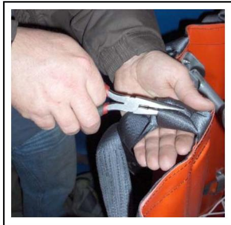
3. Holding the pliers tight, turn your hand clockwise. Repeat the operation until the knot is loose enough to remove the strap.
