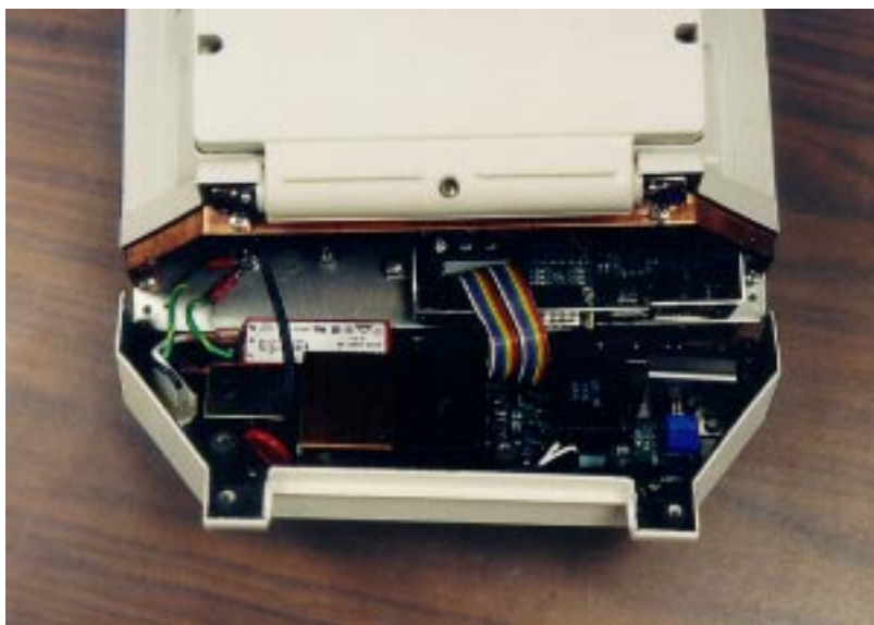
Figure 4-5 Power Supply – Partially Detached
