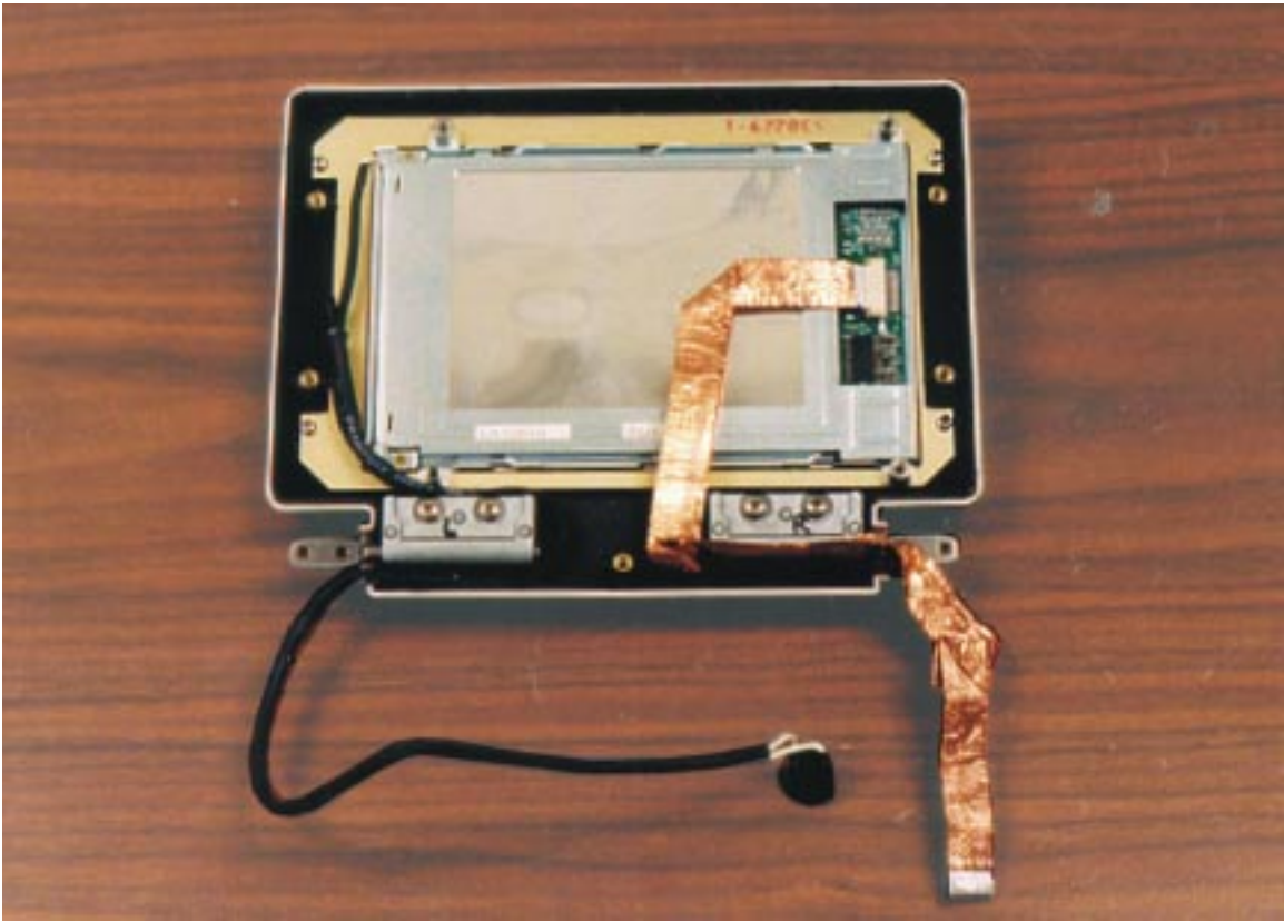
Figure 5-8 Flex Cable Replacement
