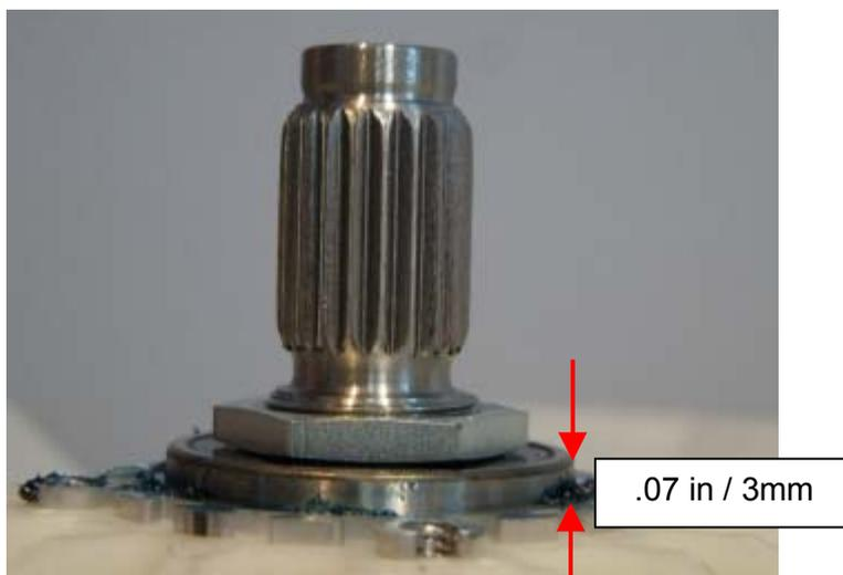
**Note:** The outer bearing will be proud of the housing by approximately .07in /3mm.
