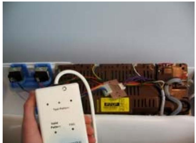
**Note: This tester does not test all the functionality of the RPS. It tests the 3 outputs but cannot indicate all faults, for example if a capacitor on the RPS is cracked.**
