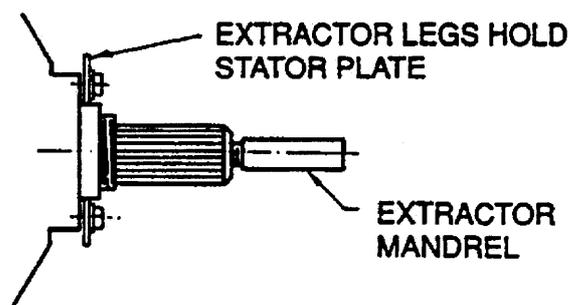
**WARNING:** Make sure the Stator clamp plate is flat before reusing. If in doubt, replace.
