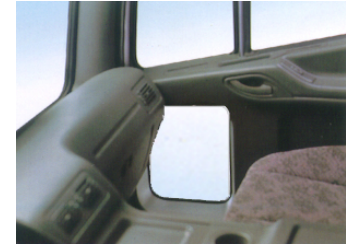
Safety window on door
