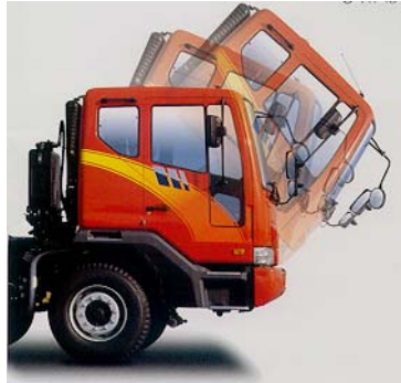
Tilting Cab up to 52 degrees
