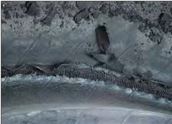
Inner liner damages
