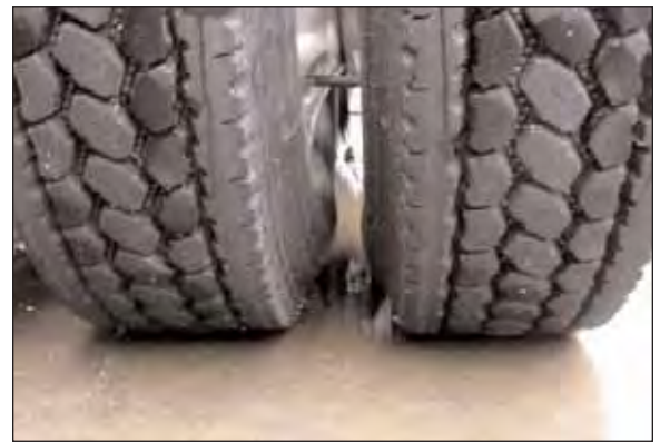
Inside dual (left) at 30 psi and outside dual (right) at 90 psi
