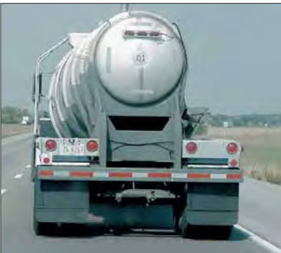
This driver has to constantly counter-steer to the left to keep the trailer off the shoulder.
