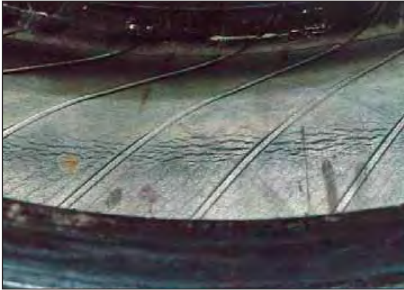
Potential zipper rupture
