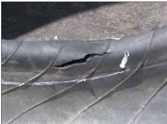
Bead damage caused by mounting/dismounting
