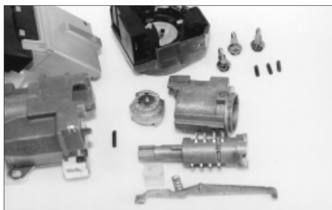
7. The entire disassembled ignition.
