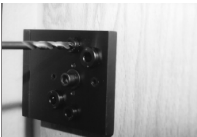
5. Now drill, using the correct guide holes for the lock.
