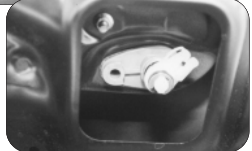
11. The trunk lock is actually part of the deck lid. Simply remove the linkage rod and 10mm bolt to remove it.
