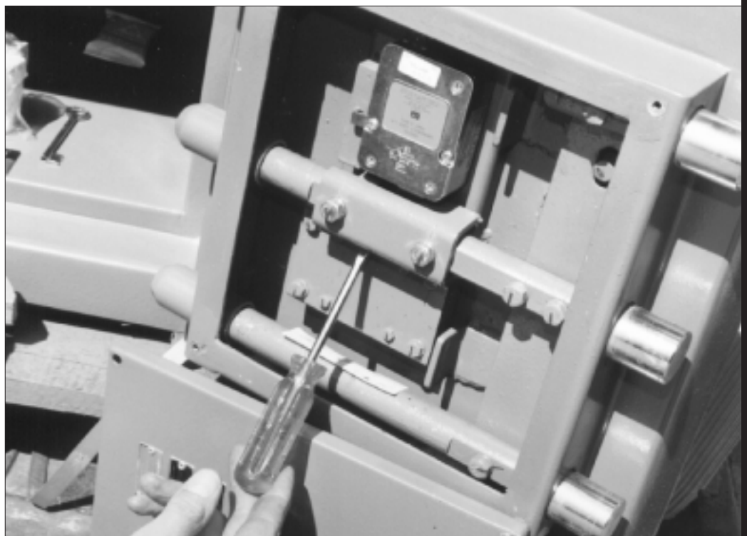
7. Inside of door showing the three active one-stage locking bolts. The screw driver is pointing to the key lock which is mounted VU.
