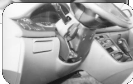
2. This column uses a two piece clam-shell shroud, held together by six screws.
