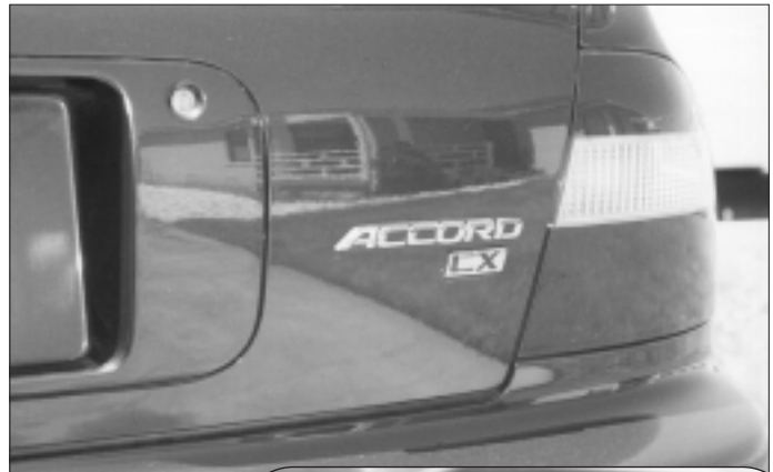
11. The trunk lock is actually part of the deck lid. Simply remove the linkage rod and 10mm bolt to remove it.
