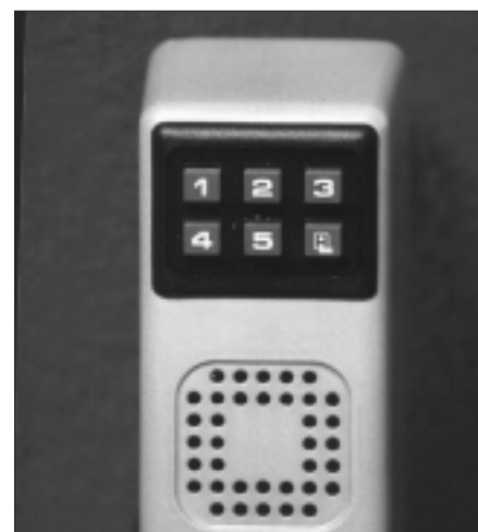
2. The PG30 is activated using a keypad instead of a key.
