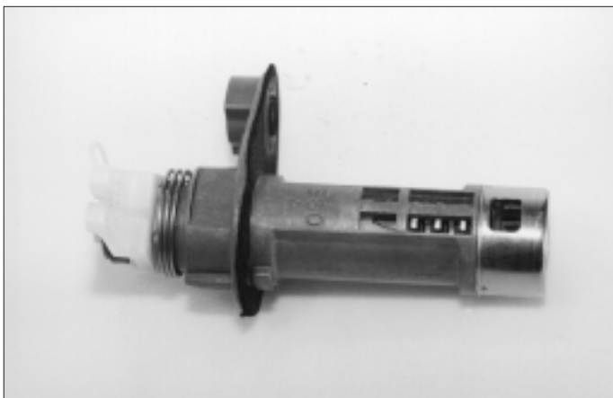
12. The face cap on this lock can be removed but must not be damaged.
