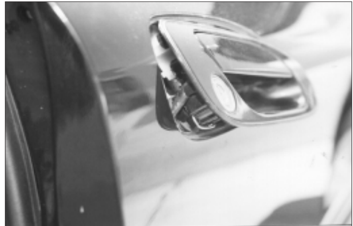
9. The handle is held to the door via two 10mm bolts. Remove them and slide the handle out the front.
