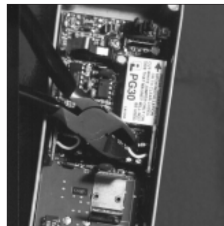
5. After choosing what side the magnet is going to be on, cut the appropriate wire.
