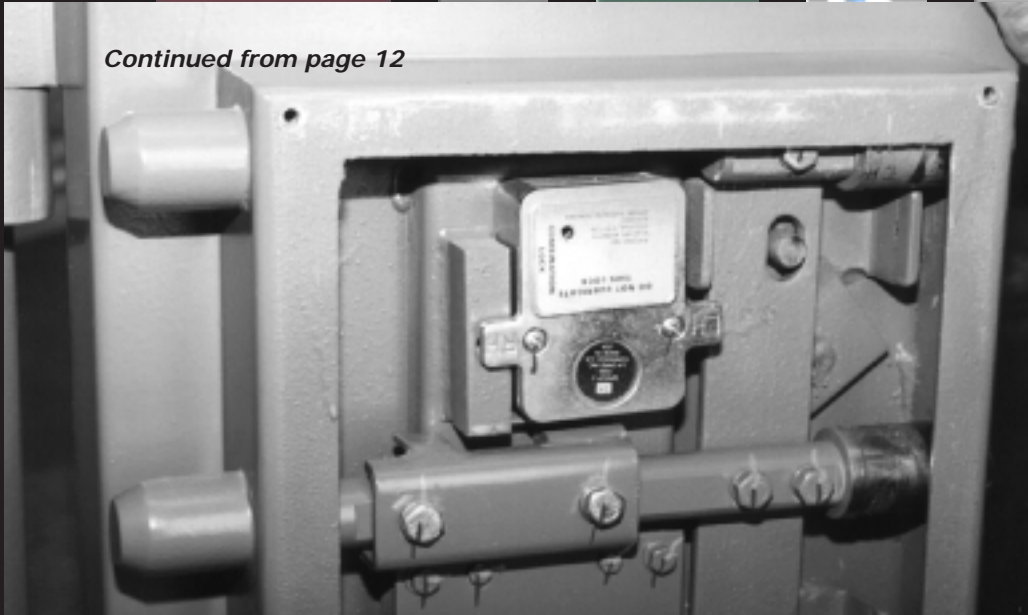
2. Mechanical Lock mounted VD with LaGard Dual relock cover. Note massive stationary bolts on hinge side of door.
