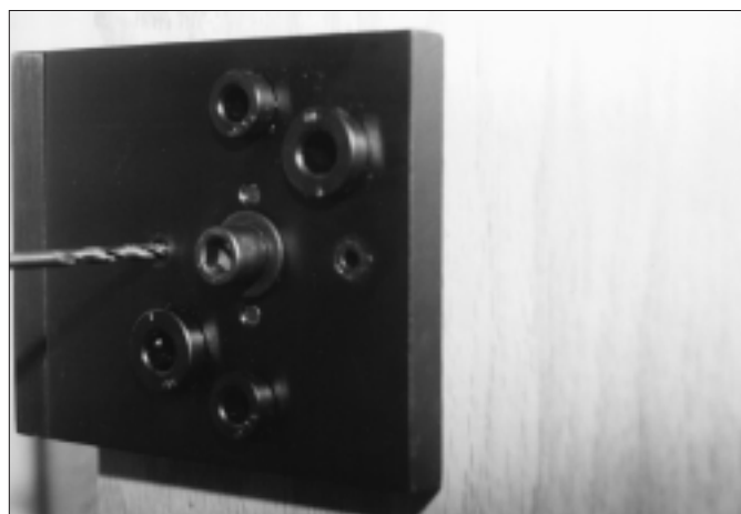
6. With the support post holes drilled, drill holes for the locator tabs.
