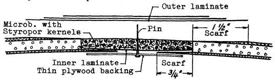
Basically it is possible to repair also larger shell parts in the foregoing manner. Because of weight you should use a plug of foam in place of the microballoons and Styropor kernels.
