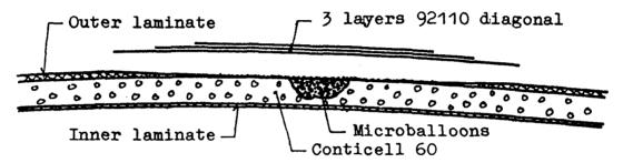
After hardening (appr. 8 hrs. at 20 deg. C. or 68 deg. F.) the damaged area should be smoothed, filled and painted. In smoothing take care that only the edges of the patches are sanded.
