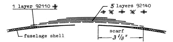
For small holes or fractures the repair is no problem. You sand your scarf, clean well with carbon tetrachloride or acetone, lay on the cloth layers and, if the resin is dry, can finish the whole repair with microballoons after 2 or 3 hours.
