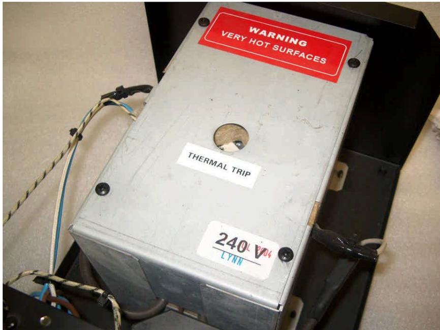
1. Always try to change a **HEAT EXCHANGE** when it is cold as the exposed metal parts can be **VERY HOT**.
