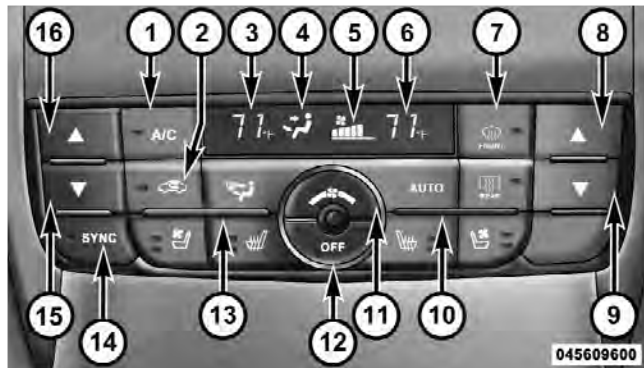
Automatic Temperature Control (ATC) Panel
